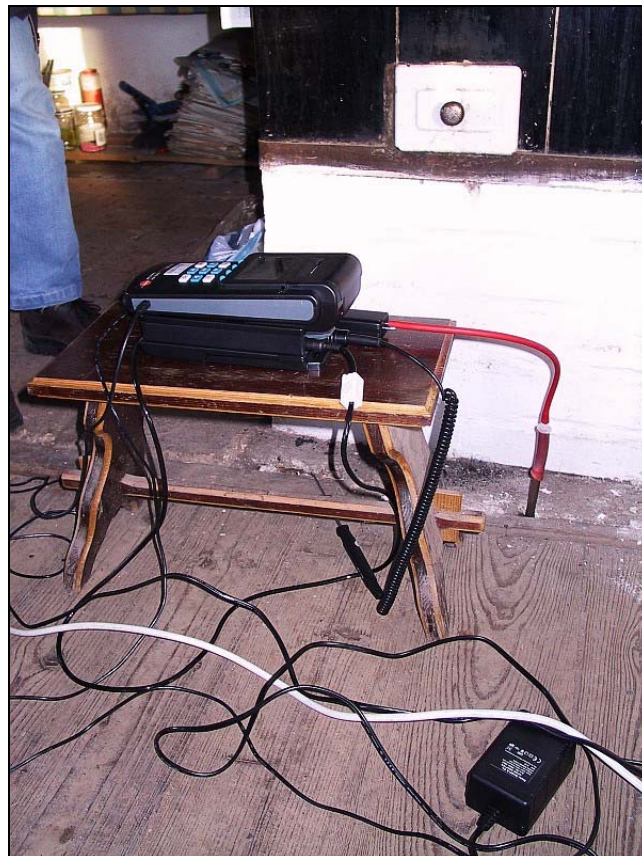
Fig. 1 - In situ measurement of air velocity and pressure difference
