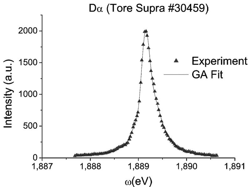
Fig. 3: Comparison of the experimental (Tore Supra shot 30459) and model profile of  $D\alpha$  for a Tore Supra configuration using the Toroidal Pumped Limiter
