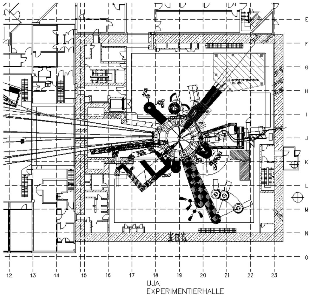
Fig. 5A: Lay-out of the experimental hall in the ground floor of the reactor building of FRM-II
