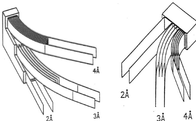
Fig. 4: Two types of beam splitters
