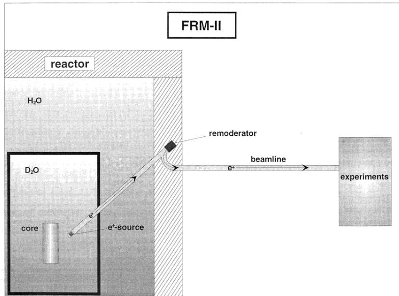
Fig. 1: Scheme of the positron source at FRM-II
