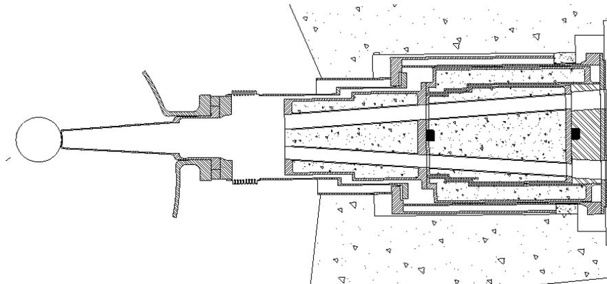
Fig.3: Principal design of a beam tube plug with 2 neutron channels and a rotating shutter
