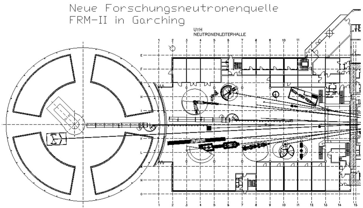
Fig. 5B: Lay-out of neutron guides and instruments in the neutron guide hall of FRM-II
