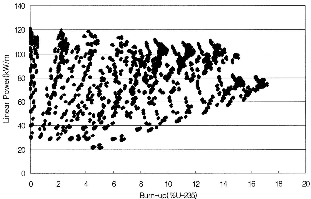
Fig. 3 Linear Power History of Full-length  $U_3Si$  Test Bundle in HANARO
