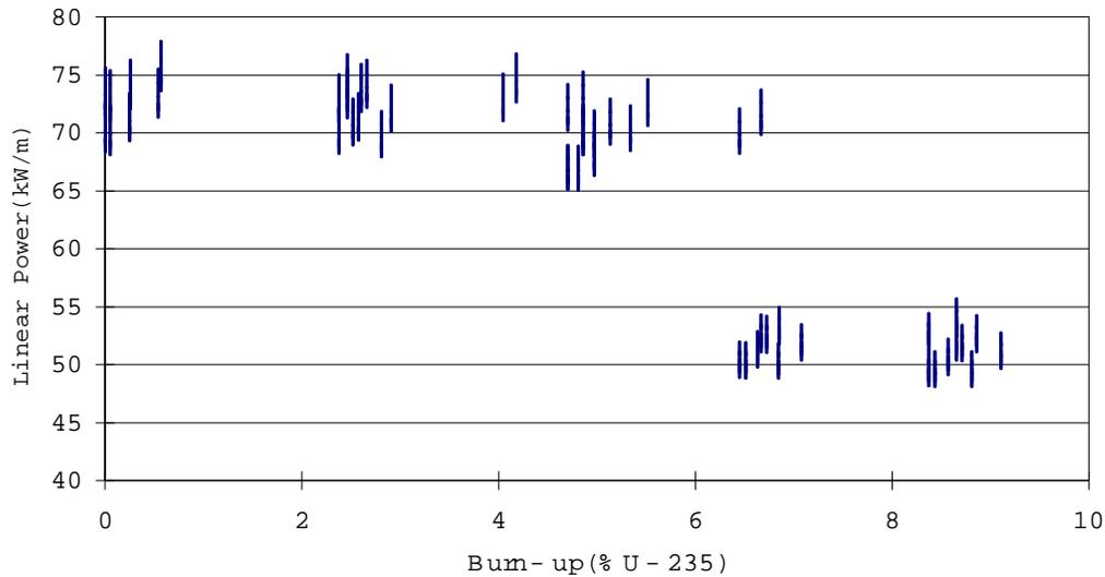
Fig. 4 Linear Power History of High-density  $U_3Si_2$  Mini-plate in HANARO
