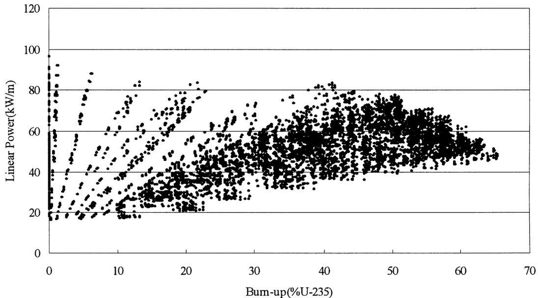
Fig. 6 Linear Power History of Type A Test Bundle-1
