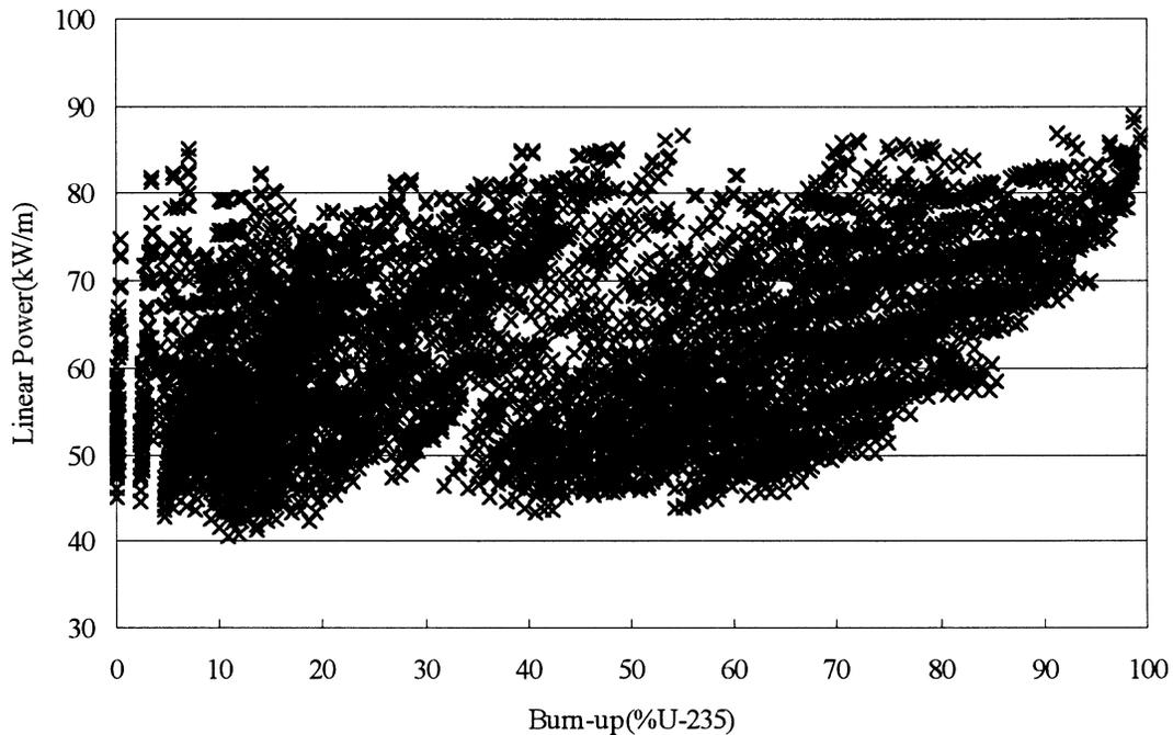
Figure 2. Linear Power vs. Burn-up of the test bundle in the core.
