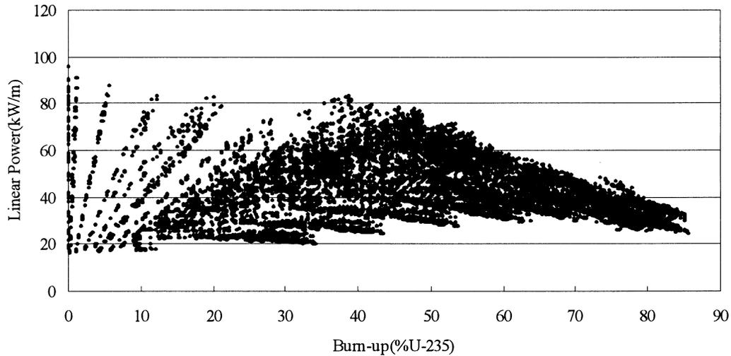
Fig. 7 Linear Power History of Type A Test Bundle-2
