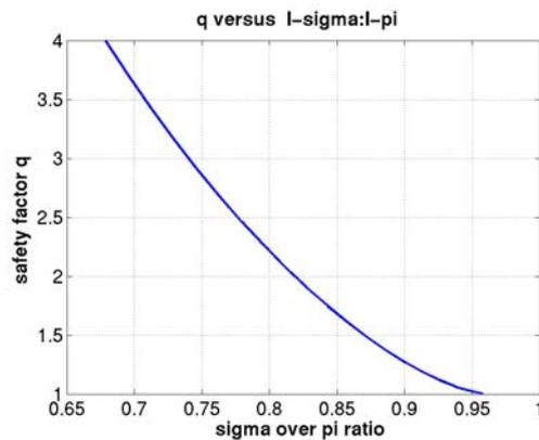
Fig3. Safety factor q versus intensity ratio of sigma & pi multiplets for lower equatorial port.
