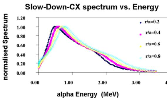
Fig.5a Predicted CX spectrum for 4 lines of sights on the HNB versus alpha energy.
