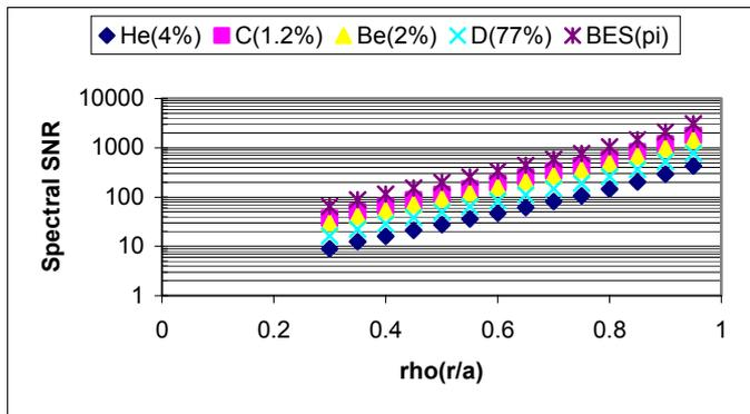
Fig.2 Expected spectral SNR ratio of the main plasma ions versus normalized minor radius. The present set assumes an offset DNB with a height of 600mm above the toroidal mid-plane. Discussions are underway for a ‘tilted’ DNB which would reach the magnetic axis.
