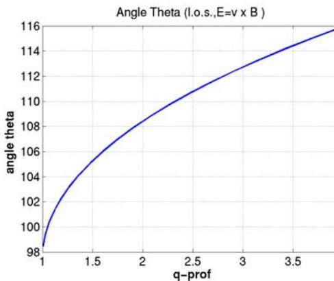
Fig2. Change of angle Theta across q-profile for lower equatorial periscope
