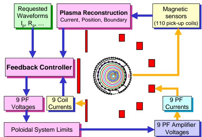
Figure 2: Current, position and shape feedback loop.
