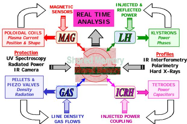
Figure 1: Tore Supra real time feedback network
