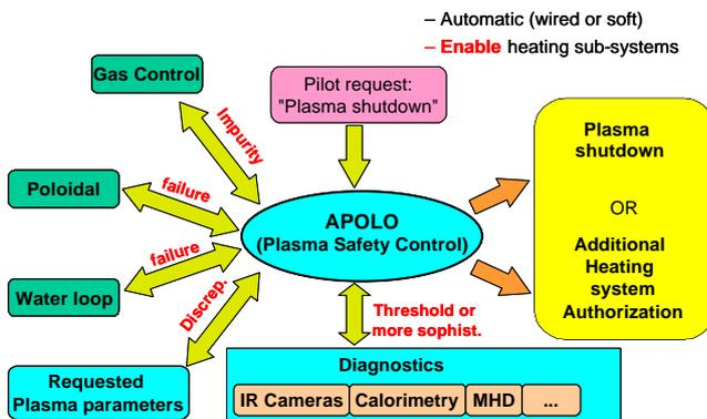
Figure 3: Plasma safety and protection system
