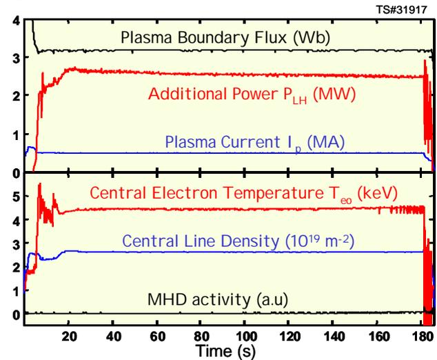
Figure 4: main plasma parameters of a 3 minutes fully non inductive discharge.
