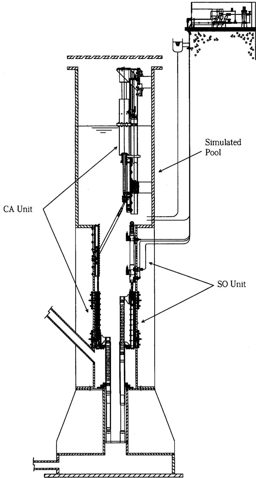
Figure 3. Concept of RCU Test Rig
