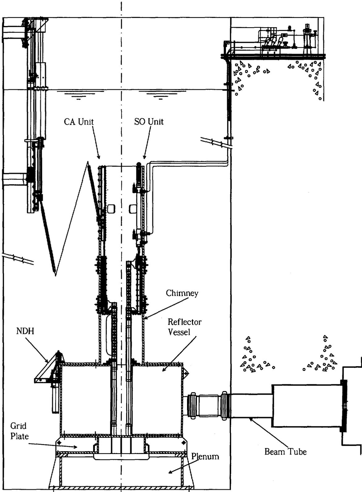
Figure 2. Reactor Structure and RCU
