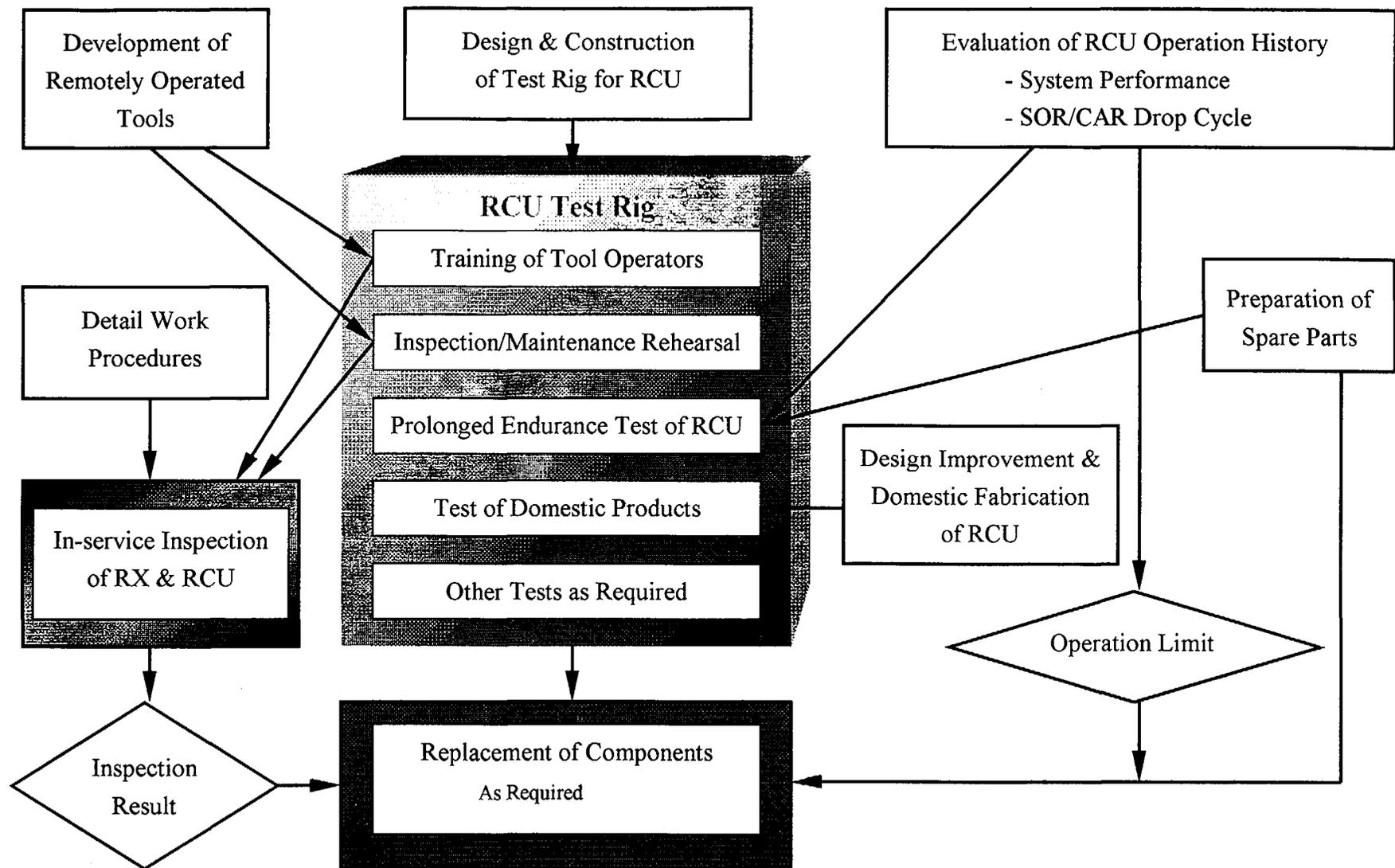
Figure 1. Flow Diagram for Inspection and Maintenance of Reactor and RCU
