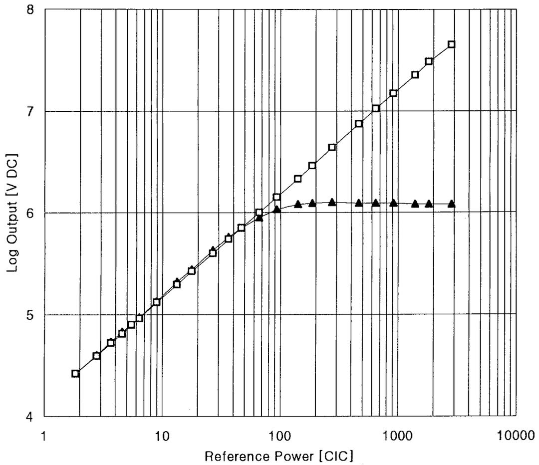
Figure 3-8 Final Results after Readjustment of LCR Gain & Zero(98.3.26 : 200W to 300KW)
