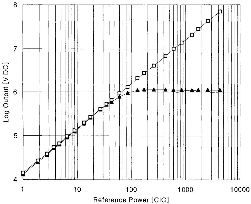
Figure 3-7 Linearity Curve after LCR Board Upgrade II(98. 3. 19 : 100W to 500KW)
