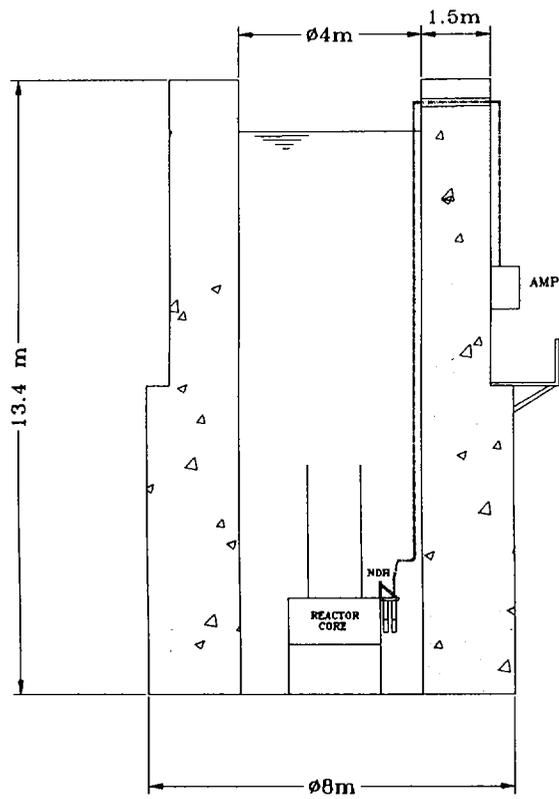
Figure 1-2 Rx Pool – Section View
