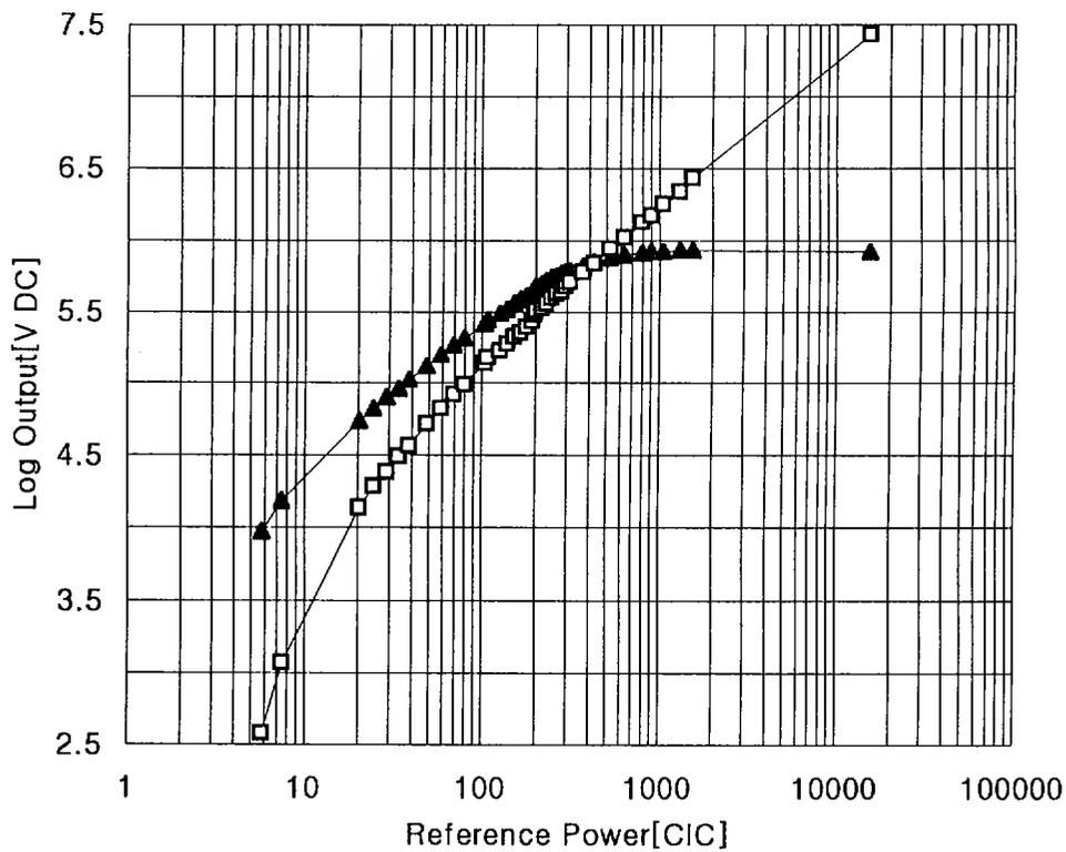
Figure 3-1 Linearity Curve for the Original System(96.9.13 : 70W to 30KW)
