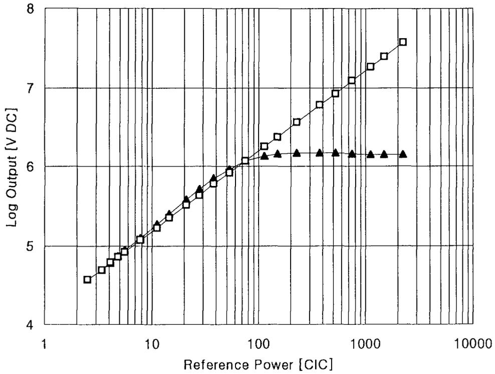
Figure 3-6 Linearity Curve after Adjustment of LCR Gain & Zero(98. 2. 11 : 300W to 300KW)
