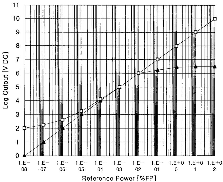
Figure 2-1 Standard Linearity Curve for WR Log Channel
