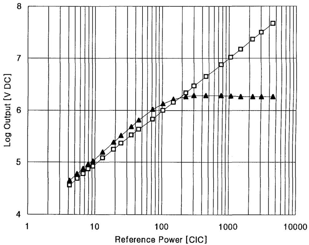
Figure 3-5 Linearity Curve after Adjustment of BP Filter Offset(97. 12. 16 : 300W to 300KW)
