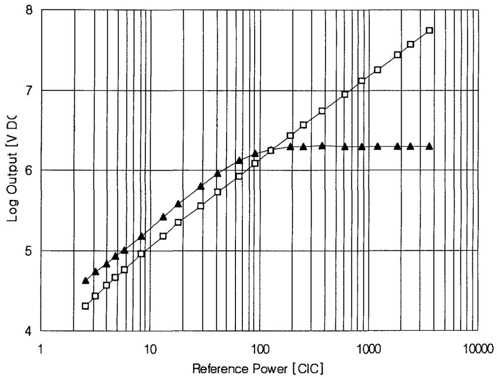
Figure 3-4 Linearity Curve after LCR Board Upgrade(97. 11. 17 : 300W to 300KW)
