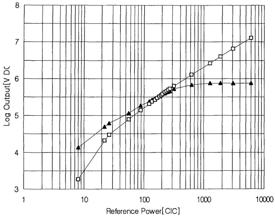
Figure 3-2 Linearity Curve after Adjustment of the MSV Gain(96. 9. 14 : 100W to 100KW)
