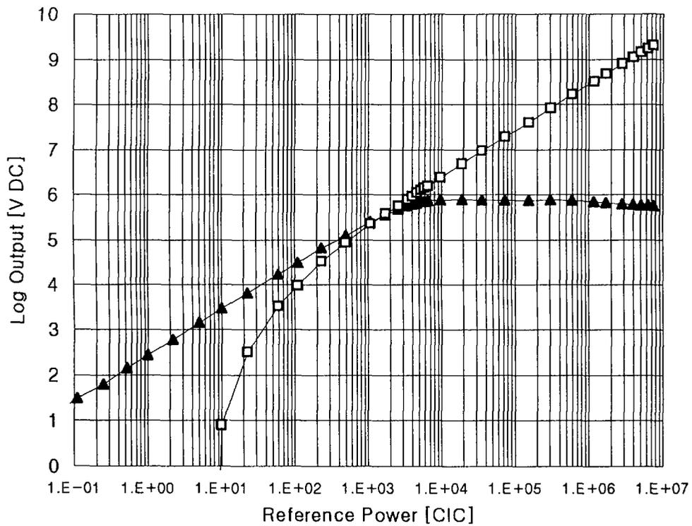
Figure 3-3 10-Decade Linearity Curve with Fresh Fuels(97. 3. 18 : 0.5W to 13MW)
