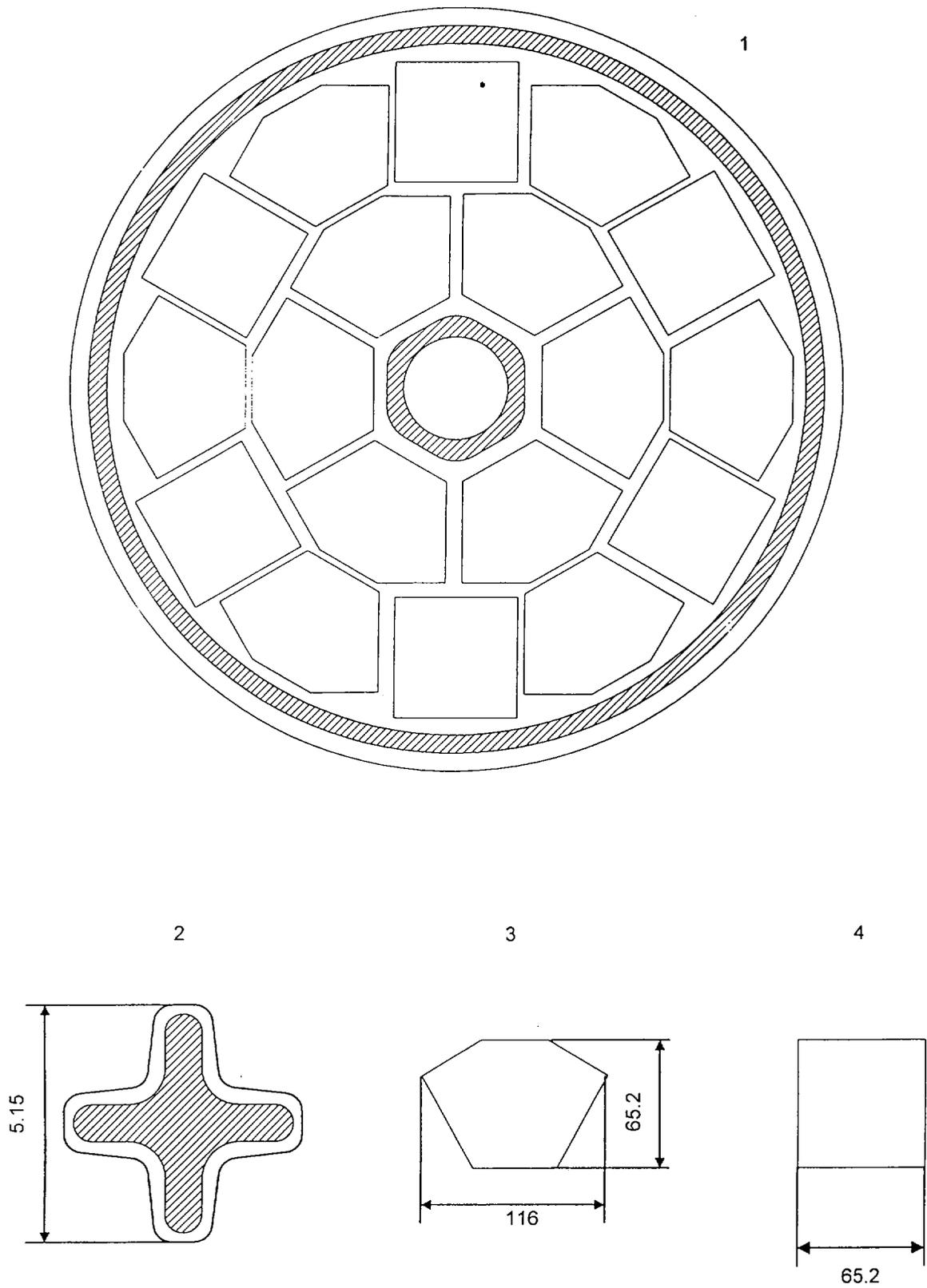
Fig. 1. PIK reactor fuel element, fuel assemble and active core
