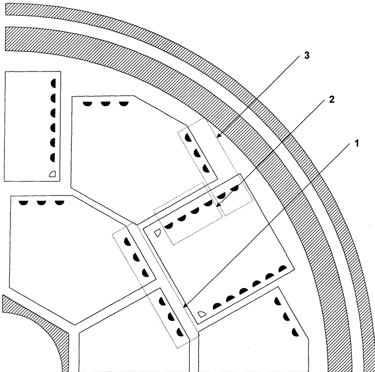
Fig.2. Burnable-absorber bar (BAB) arrangement
