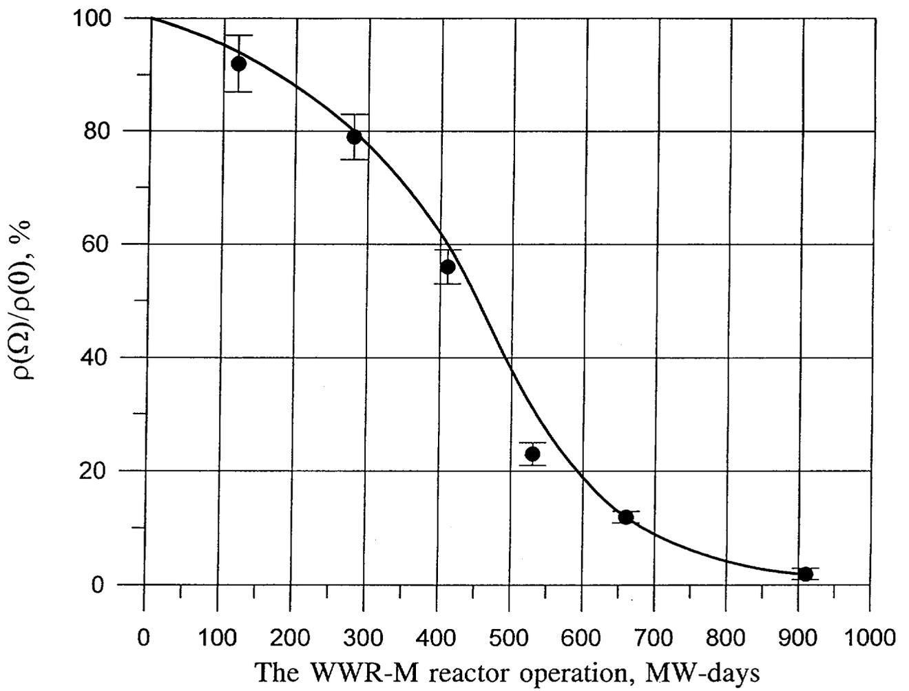
Fig.6. Ampoule relative reactivity in the course of burnup
