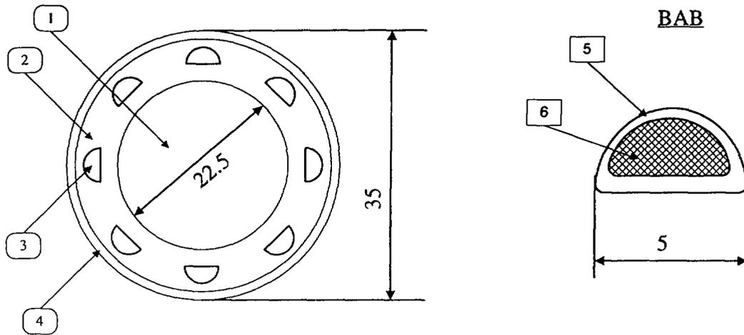
Fig.5. Burnable-absorber bar (BAB) arrangement in the WWR-M reactor ampoule.
