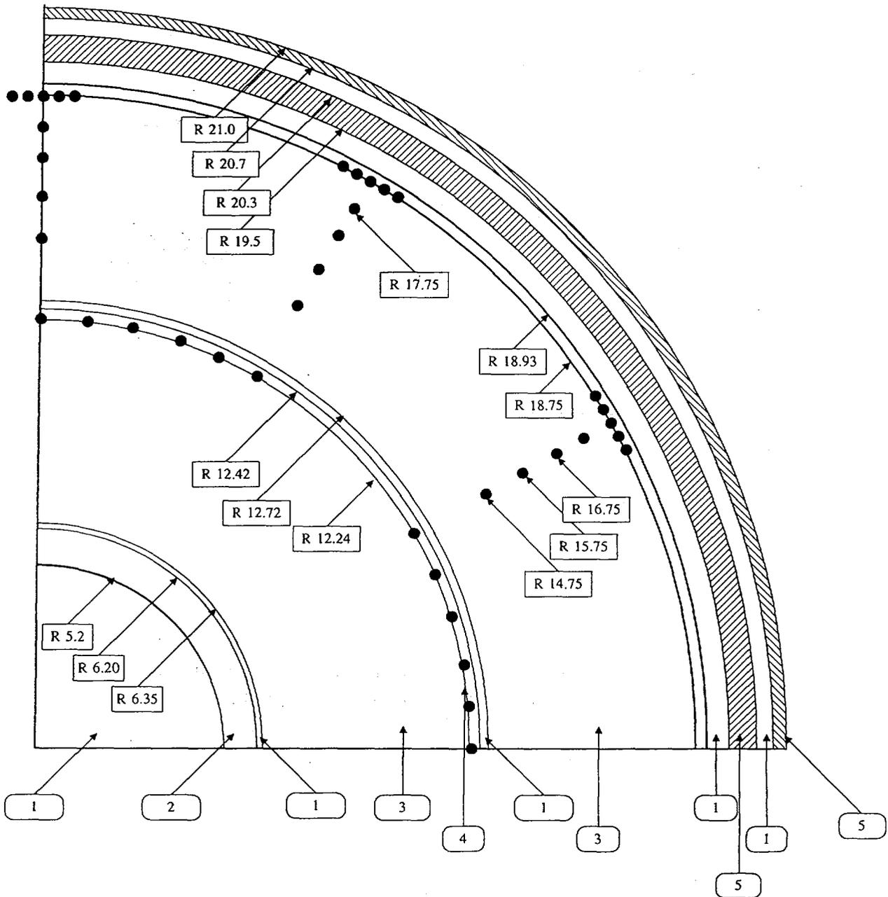
Fig.4. Burnable-absorber bar (BAB) coordinates
