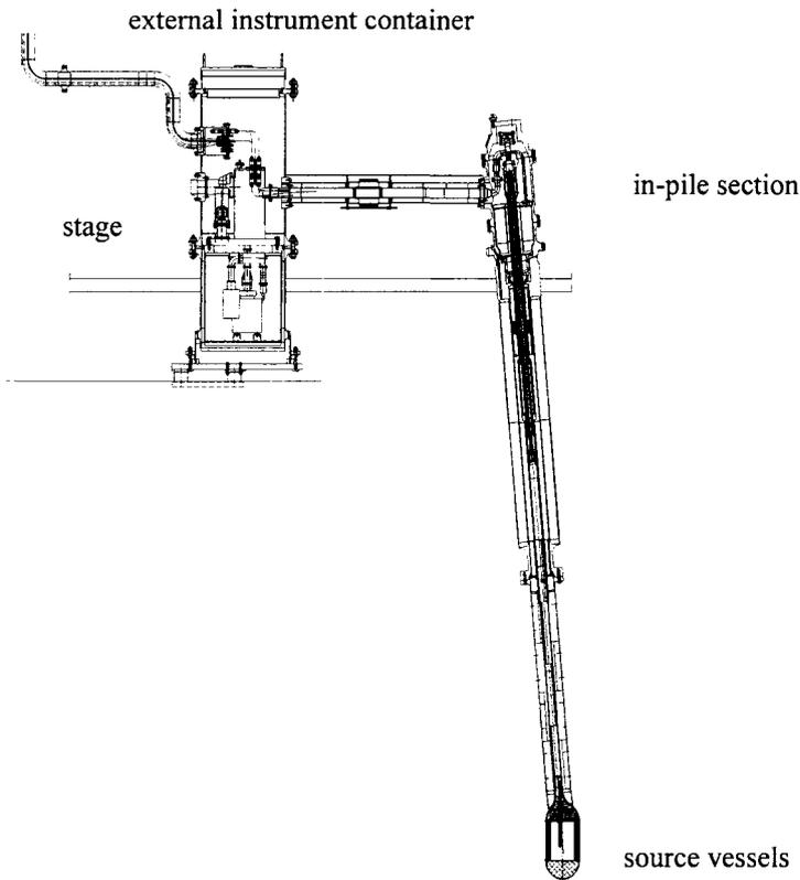
Figure 2: In-pile section and the external instrument container of the HNS
