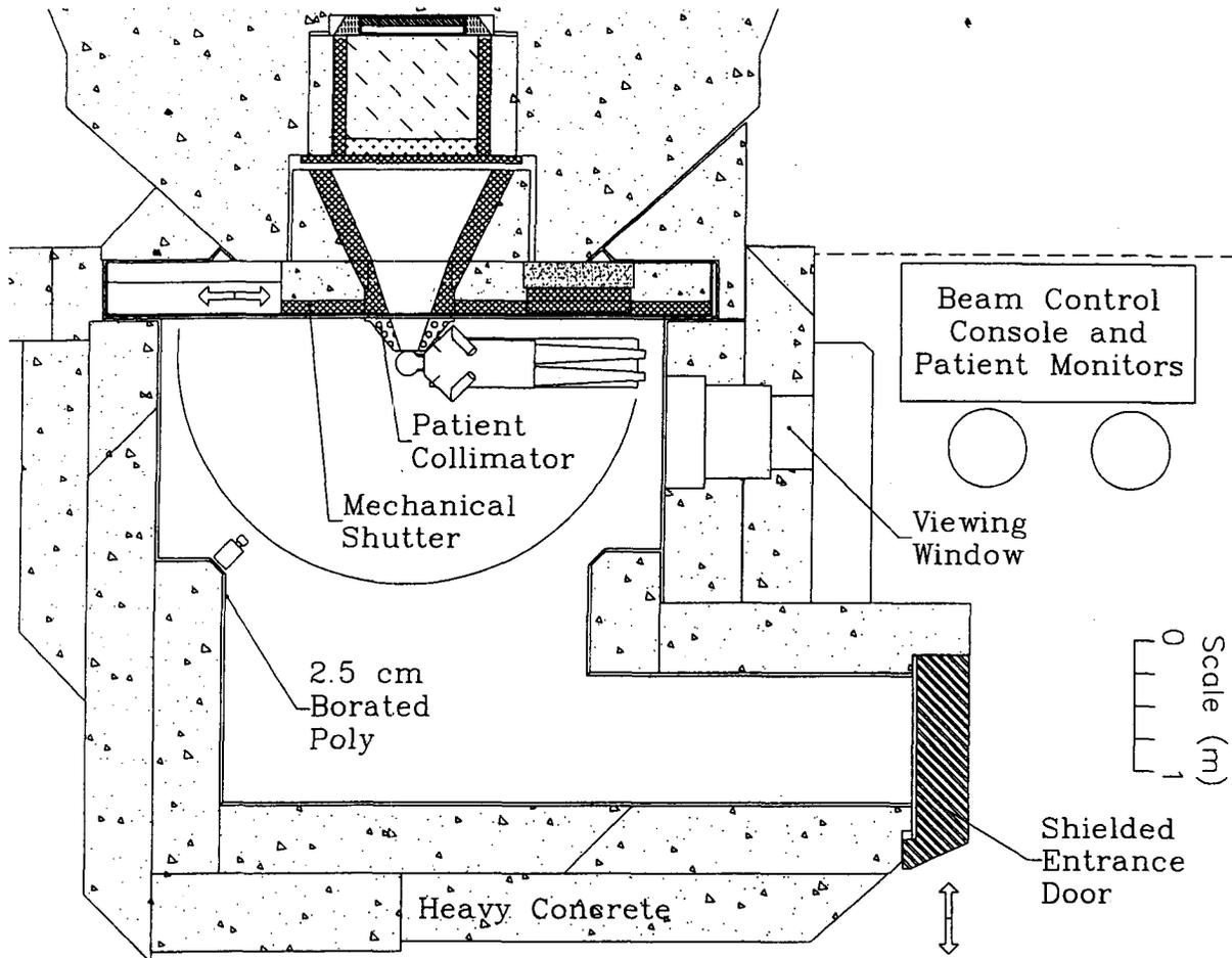
Figure. 2 Irradiation room of the MIT FCB.
