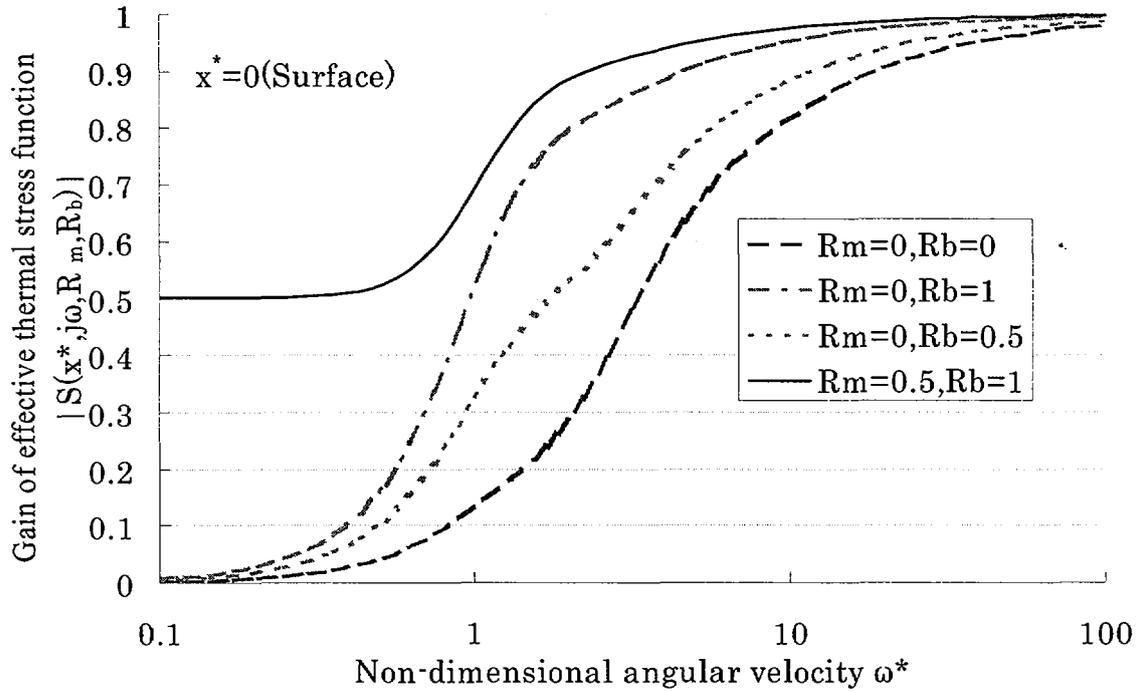
Fig.5 Effective thermal stress function:  $S(x^*, j\omega, R_m, R_b)$
