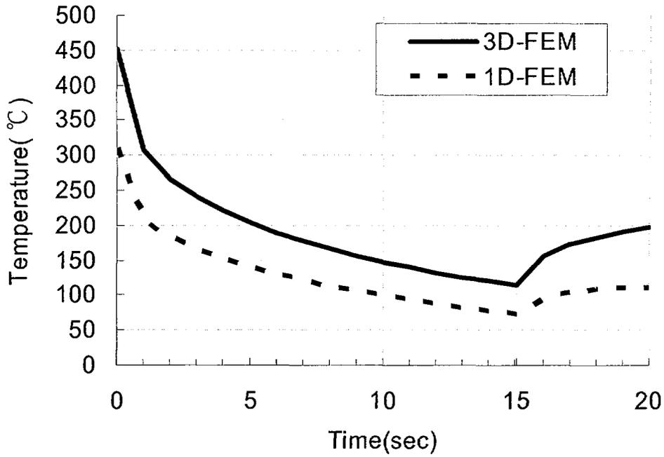
Fig.11 Temperature profile at the inner surface
