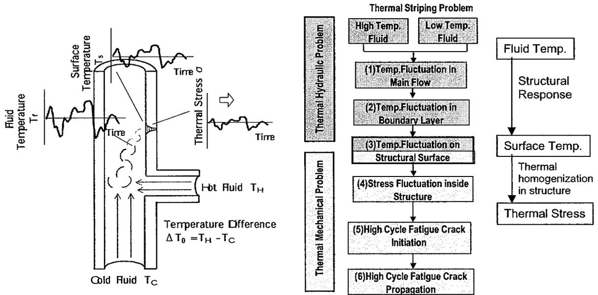
Fig.1 Thermal stripping phenomena
