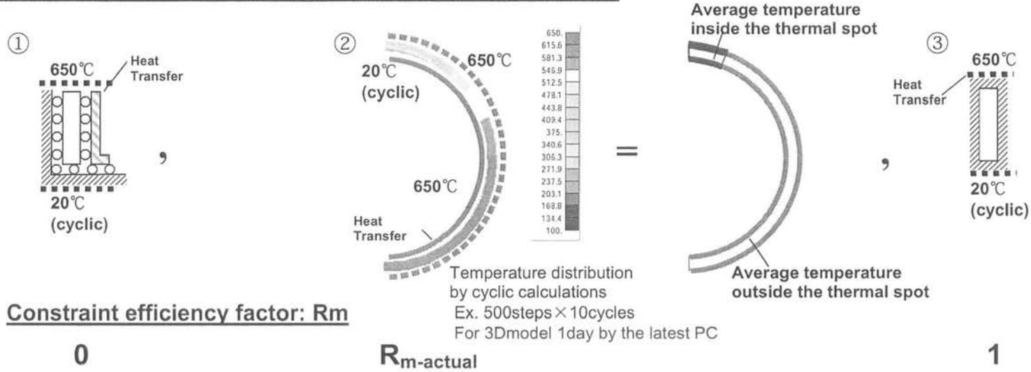
**1 step stress calculation with simplified temperature distribution**
