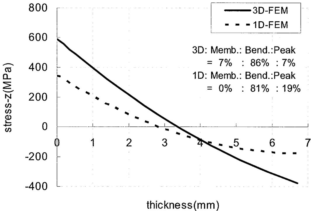
Fig.14 stress distribution in the wall : Axial
