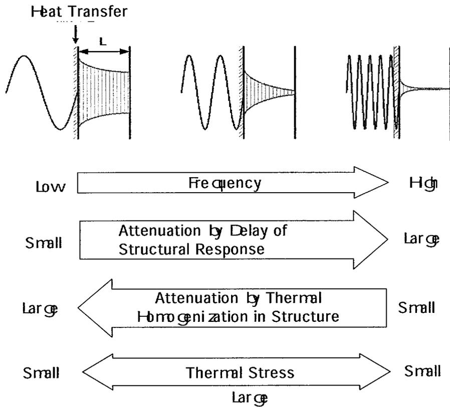
Fig.2 Frequency response characteristics of structural by fluid temperature
