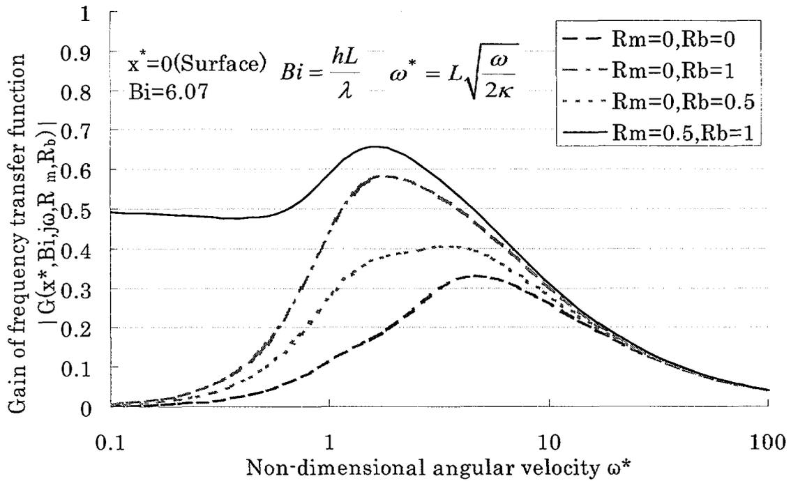
Fig.6 Frequency transfer function:  $G(x^*, Bi, j\omega, R_m, R_b)$
