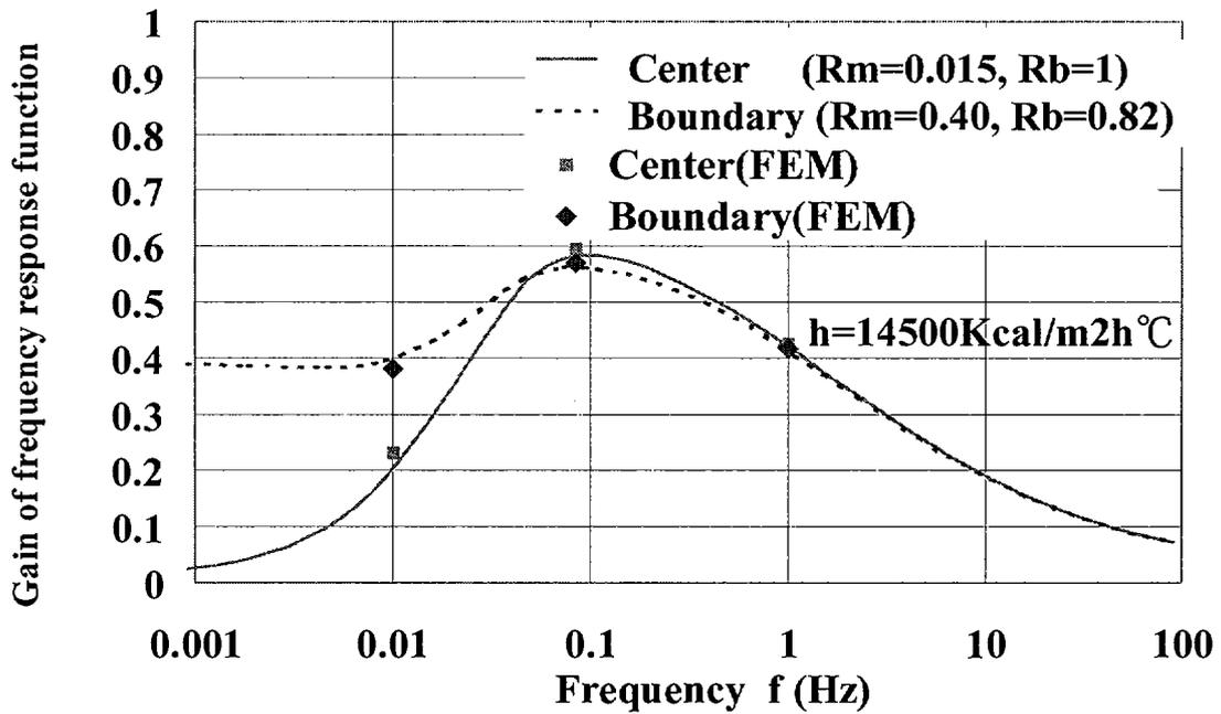
Fig.24 Frequency Transfer Function model and FEA results
