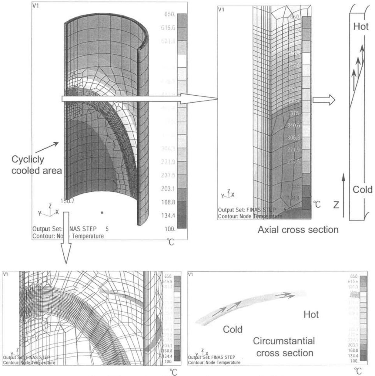
Fig.9 Example of the membrane constraint
