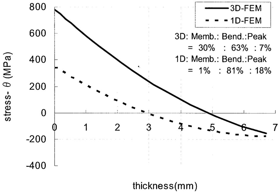
Fig.13 stress distribution in the wall : Circumferential
