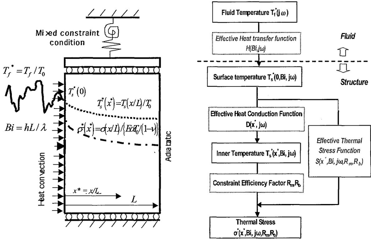
**Fig.3 Thermal and mechanical model of structural response by fluid temperature**
