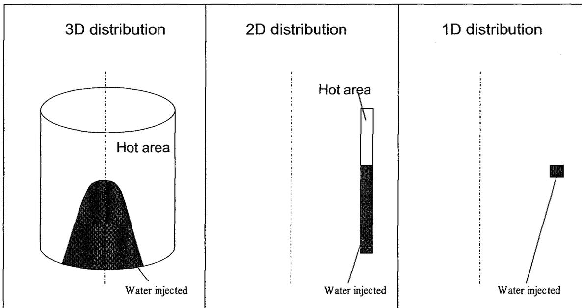
Fig.8 Example of thermal distributions: Cold spot
