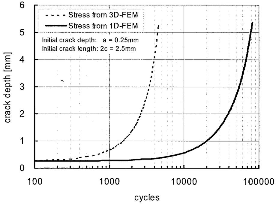
Fig.17 Crack propagation: crack depth
