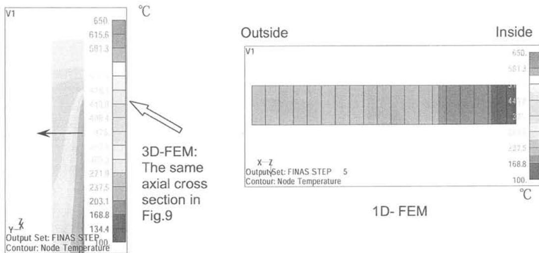
Fig.10 Temperature distribution in the wall at 4 seconds
