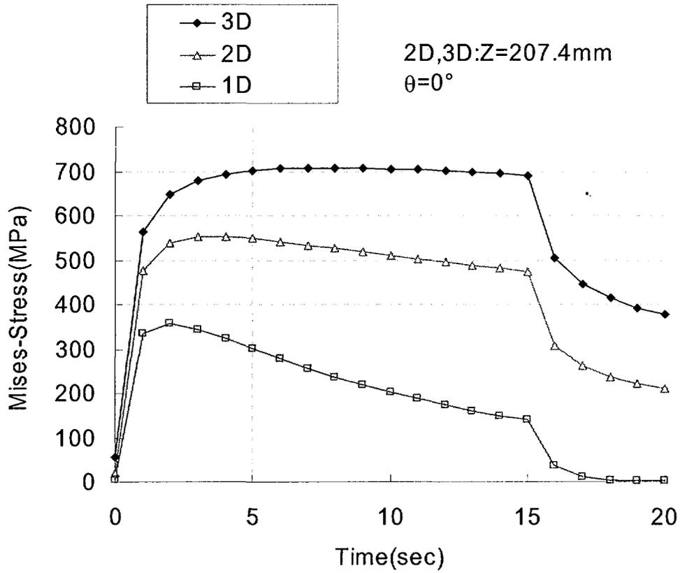
Fig.15 Von Mises stress profile at the inner surface
