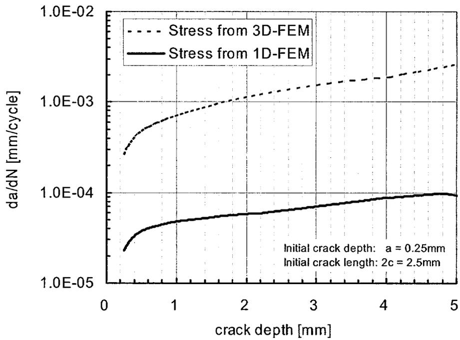
Fig.18 Crack propagation rate
