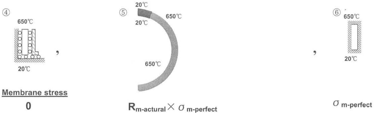
Fig.19 Membrane constraint efficiency factor
