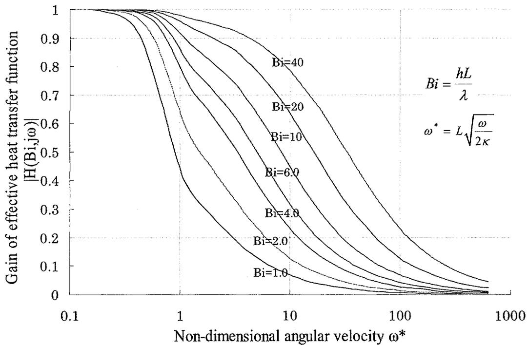
**Fig.4 Effective transfer function:  $H(Bi, j\omega)$**
