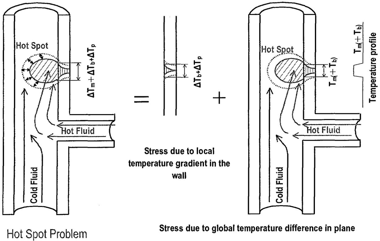
Fig.7 Temperature difference in 3D thermal distribution
