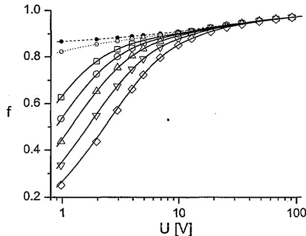
Fig. 2. Saturation curves of the REM-2 chamber, measured at different dose rates (open polygons). The values of  $f_d f_i$  obtained from the fit to Eq. 9 - (the lines in Fig.1) are depicted by small open circles and dotted line, and the finally calculated values of  $f_i$  are marked by black circles and dashed line. The solid lines were generated as  $f = f_d f_v f_i$  for each dose rate using the interpolated values of  $f_i$  - dashed line.
