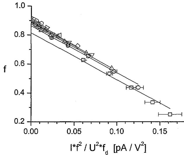
Fig. 1. Ion collection efficiency measured at different dose rates, plotted versus  $I_s f^2 / U^2 f_d$  and fitted with the set of straight lines which corresponds to certain values of the polarising voltage  $U$  - from 1 V (bottom line) to 12.7 V (upper line).
