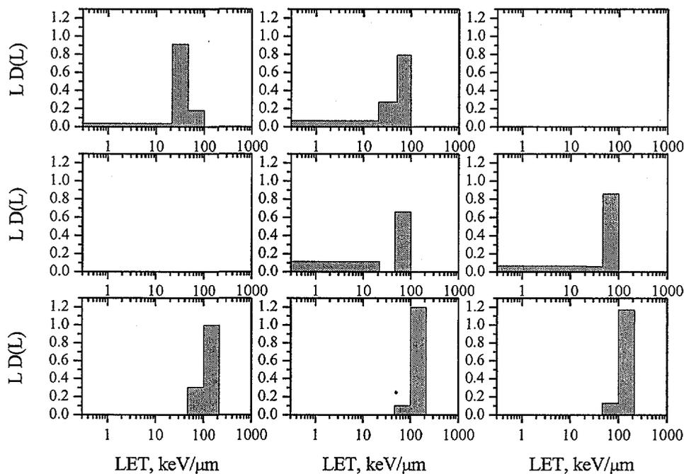
Fig. 3. Dose distributions versus restricted LET. Results for different gases are arranged in rows (TE gas, nitrogen and  $^{10}\text{BF}_3$  from the top to the bottom). Results for different radiation fields are shown in columns (bare source, the source in paraffin filter and in iron filter – from the left to the right).
