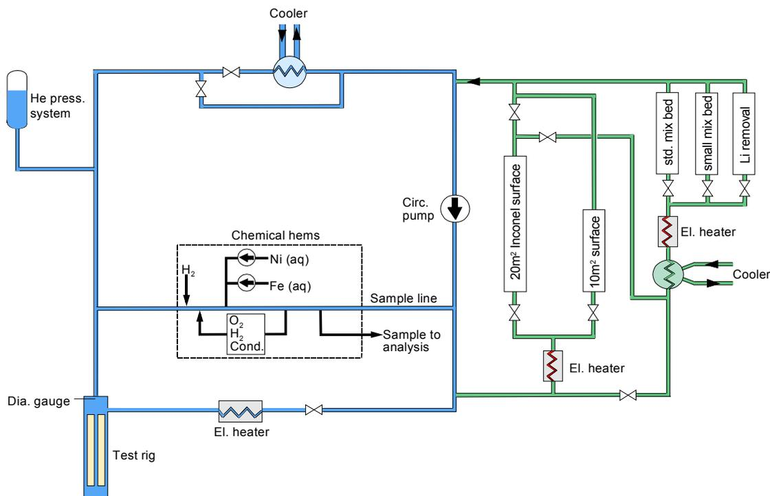
Figure 2. Schematics of a PWR loop for crud/AOA studies
