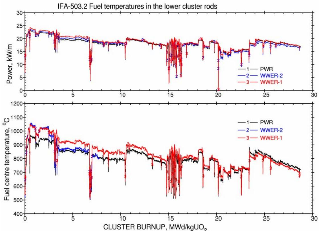
Figure 6. Development of fuel temperature in WWER and reference fuels
