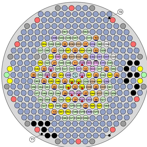
**Figure 1. Cross-section of the Halden reactor core. Of more than 300 individually accessible positions, 100-110 in the central area are utilised for fuel elements. This increases the power density and protects the pressure vessel from radiation. 30-35 experiments can be served at the same time.**
