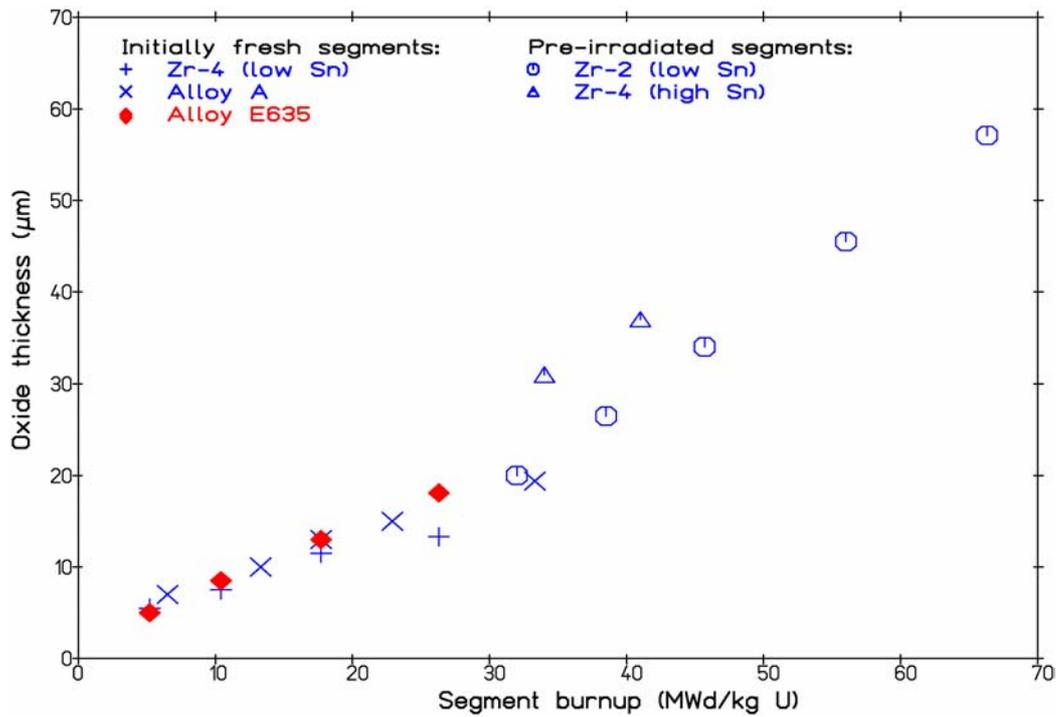
Figure 7. Oxide thickness growth of Alloy E635 under PWR conditions; comparison with Zry-2 and Zry-4 with low and high Sn content
