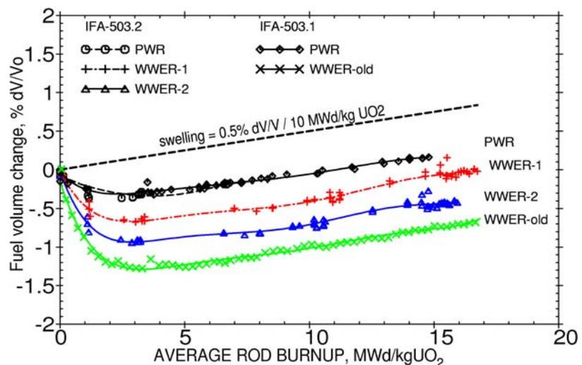
Figure 5. Densification and swelling behaviour of modified WWER fuel in comparison with old fuel types
