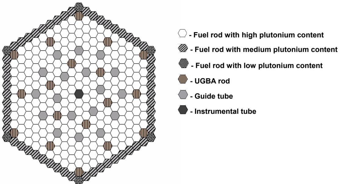
**Figure 7. The pattern of the typical MOX FA**
