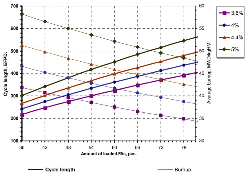
Figure 2. Cycle length and fuel burnup versus fuel enrichment and amount of loaded FAs
