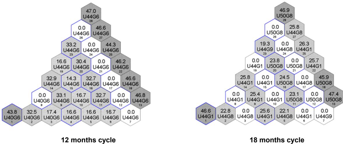
Figure 4. Loading patterns of equilibrium cycles with low leakage
