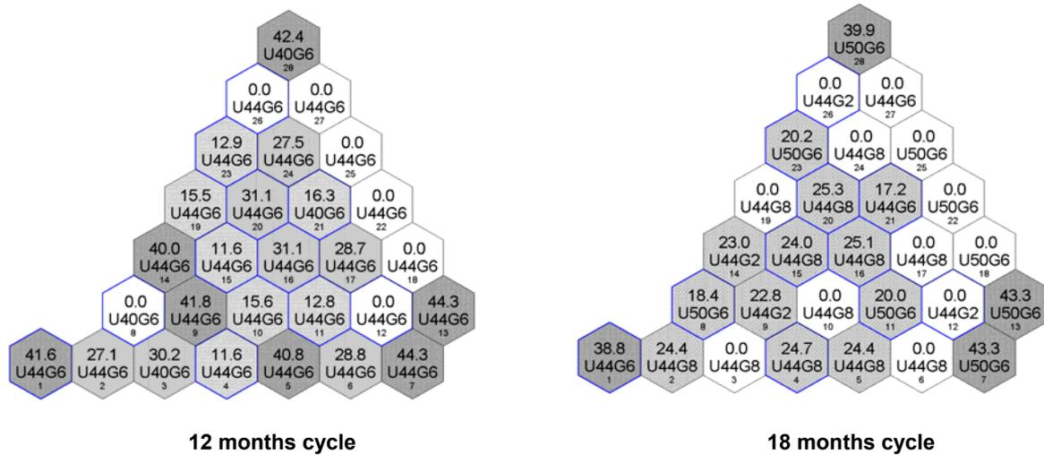
Figure 3. Loading patterns of equilibrium cycles with reduced leakage
