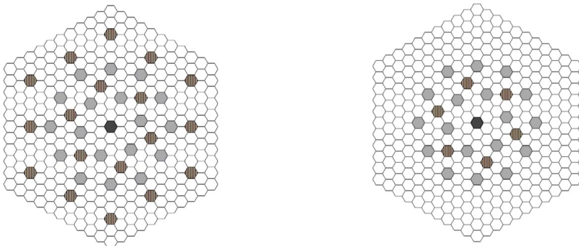
Figure 1. Arrangement of rods within fuel assemblies
