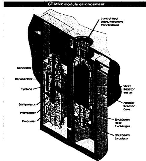
Figure 8. Main Components in GT-MHR
