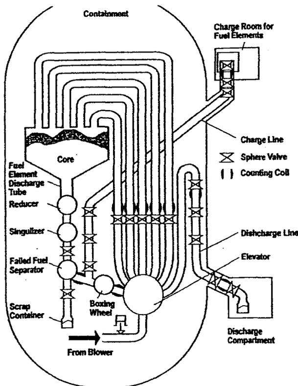
Fig. 1 MPBR cross section
