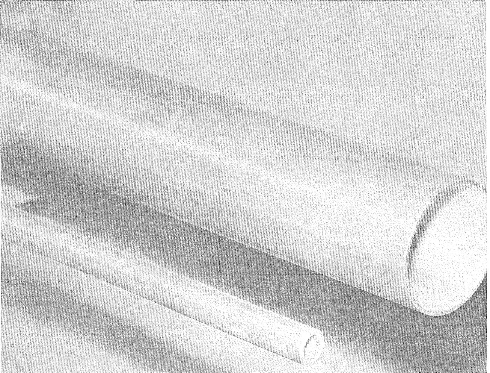
FIGURE 6. Small-Scale and Full-Size Outer Fuel Tubes
