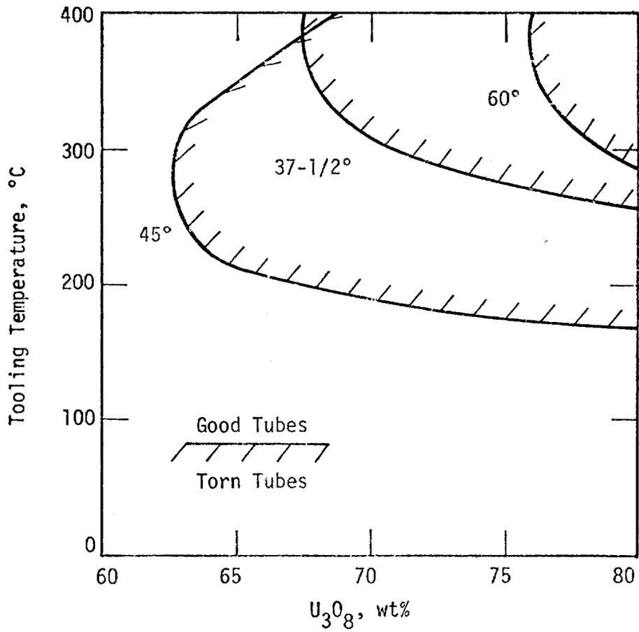
Fig. 7. Effect of U<sub>3</sub>O<sub>8</sub> Content, Extrusion Tooling Temperature, and Half the Die Cone Angle on Tube Quality.
