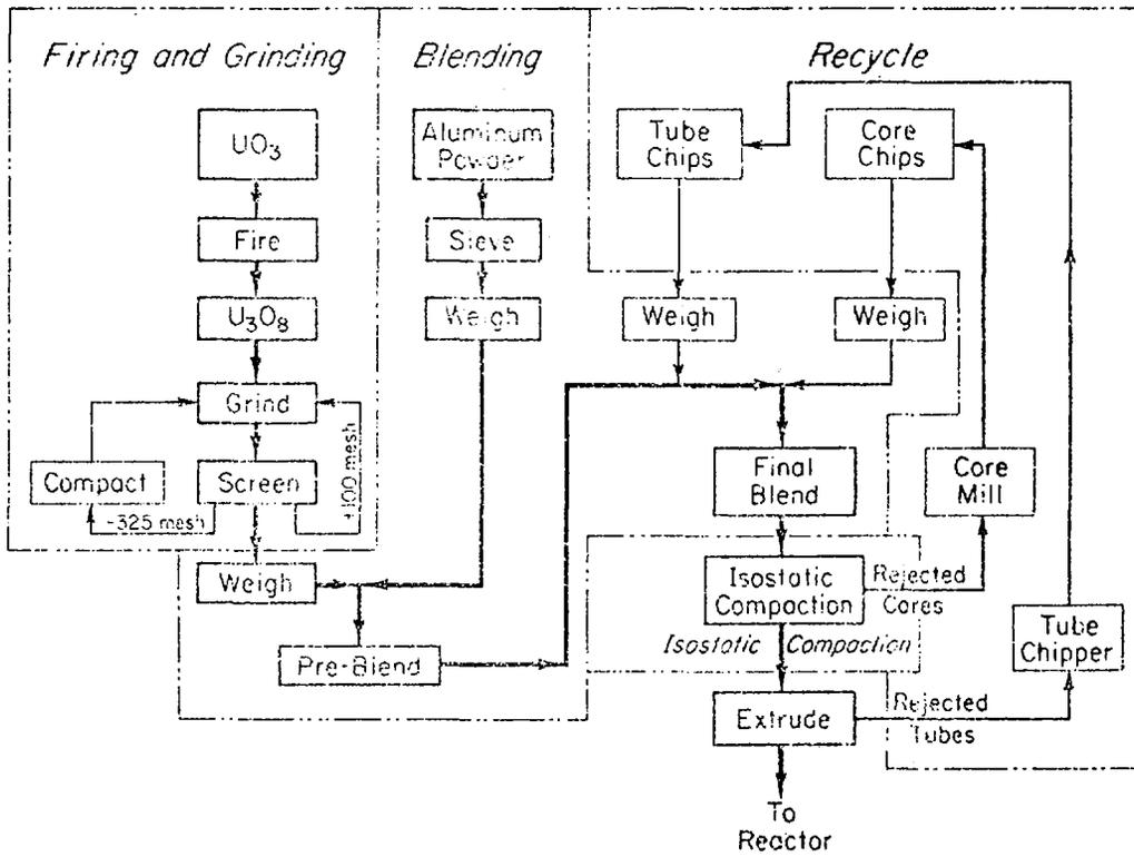
Fig. 2. Block Diagram for P/M Core Fabrication.
