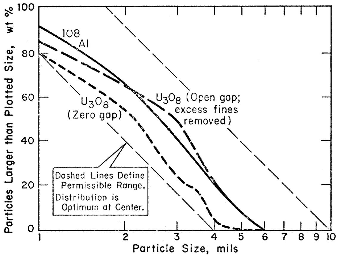
Fig. 3. Particle Size Distribution for Roll Ground U<sub>3</sub>O<sub>8</sub> and 108 Aluminum Powder.
