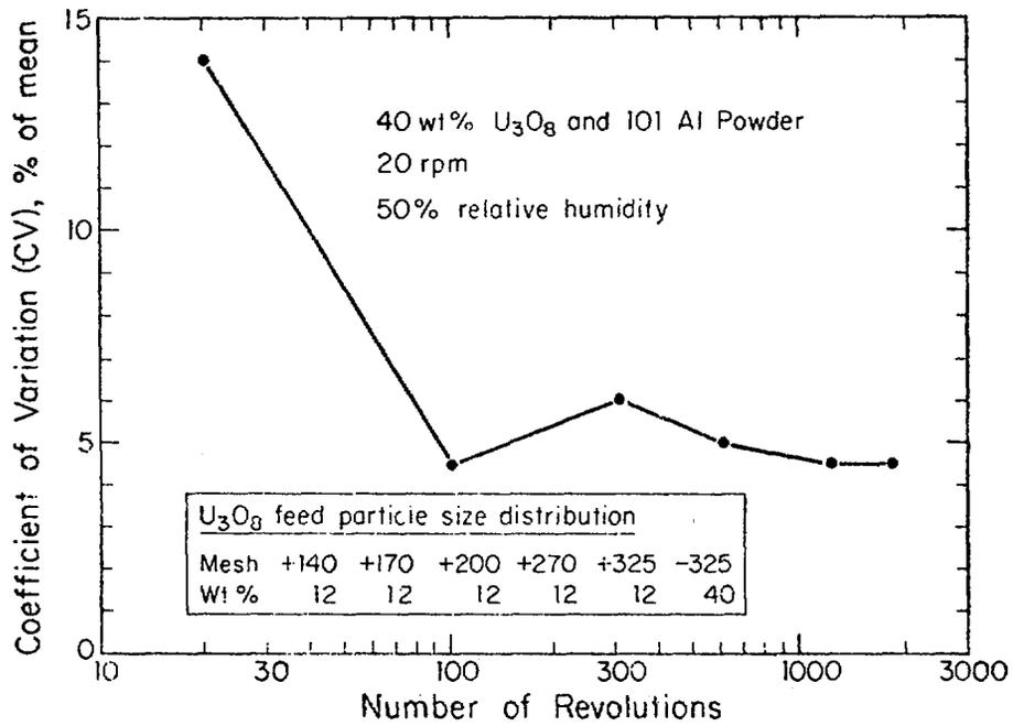
Fig. 5. Test of Modified Tumbling Mixer.
