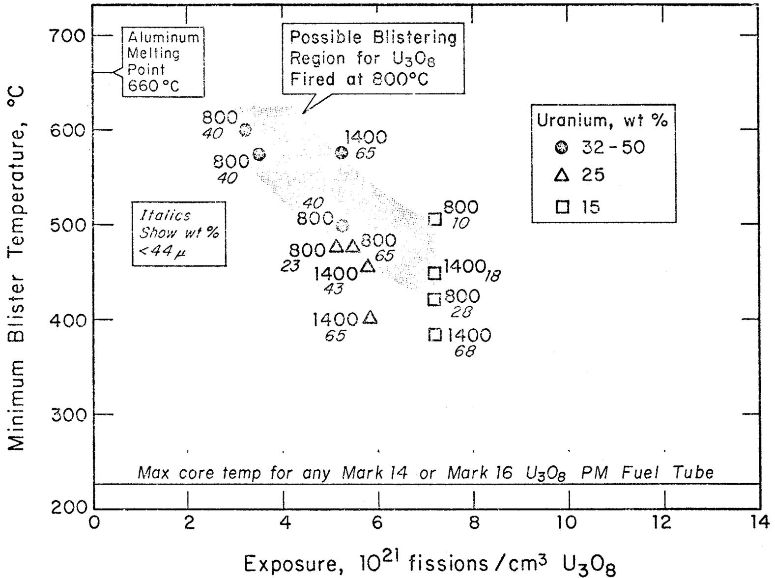
Fig. 9. Temperatures Required for Blister Formation on Irradiated Fuel Tubes with  $U_3O_8$  P/M Cores ~40% Burnup.
