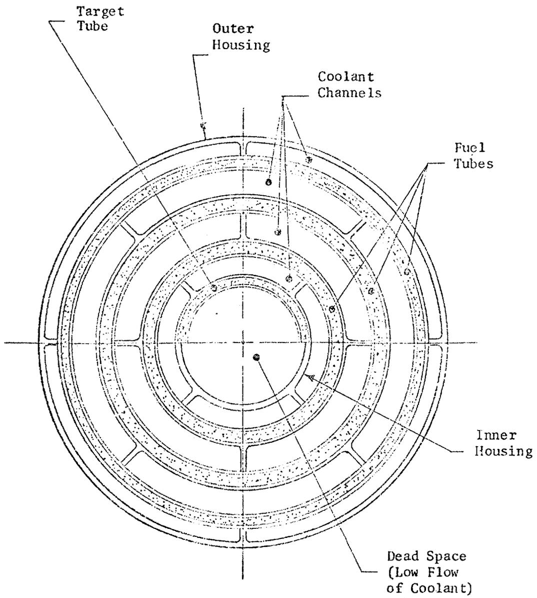
Fig. 1. Cross Section of a Fuel Assembly
