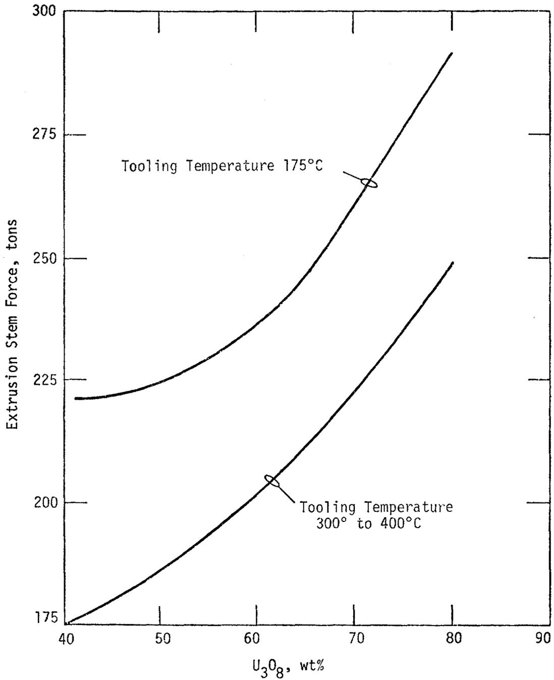
Fig. 8. Effect of Tooling Temperature and  $U_3O_8$  Concentration on Extrusion Force Required.
