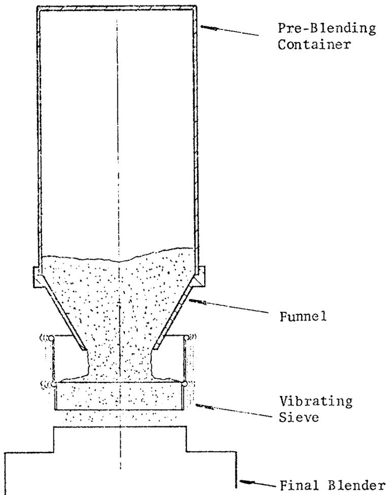
Fig. 4. Powder Pre-Blend and Sieving Apparatus
