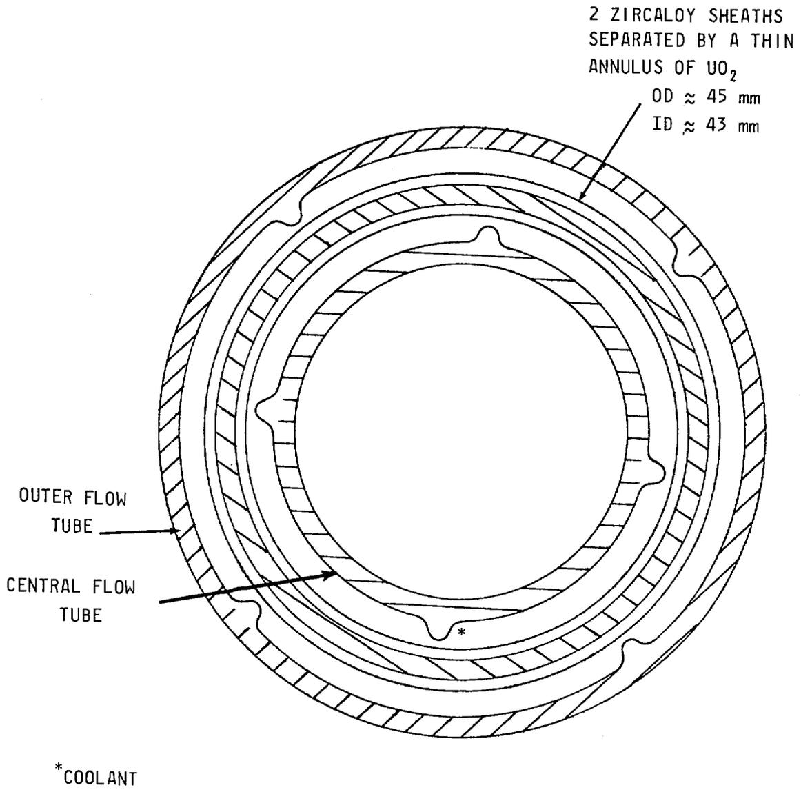
Fig. 4 Mark 7 ( $UO_2$ ) Fast Neutron Rod for NRX Reactor
