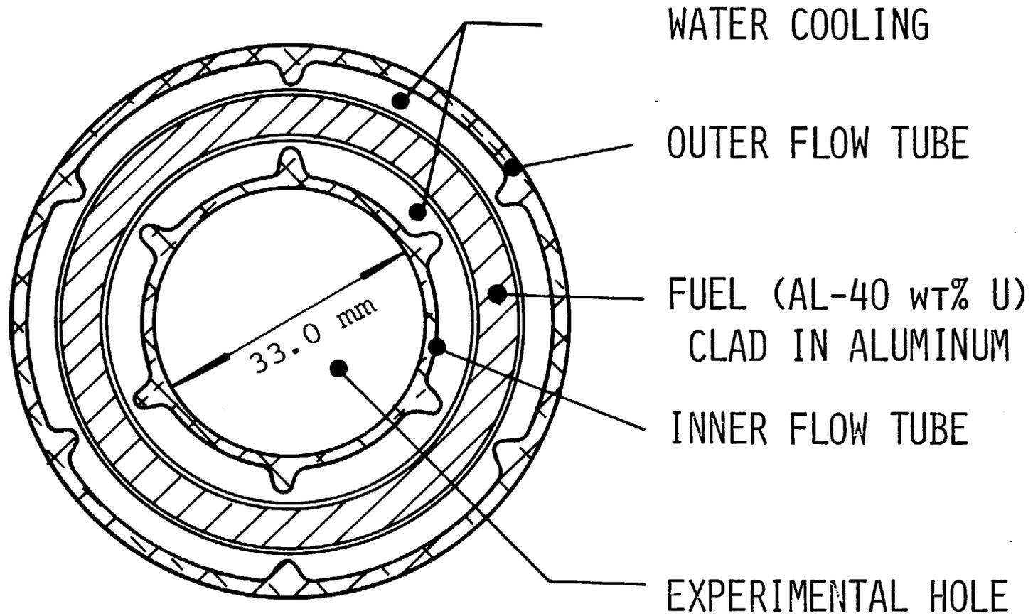
Fig. 3 Mark 6 Fast Neutron Assembly (NRX)
