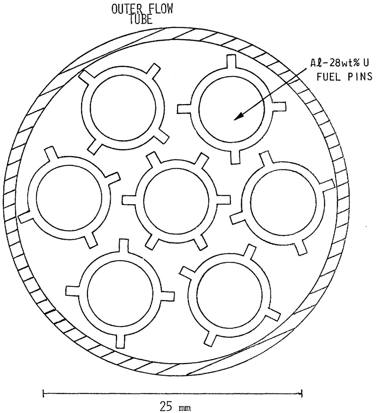
Fig. 1 Seven Element U-Al Rod Design for NRX
