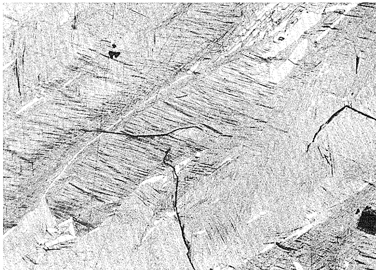
Fig.2: Microstructure of U_6Fe after heat treatment.
