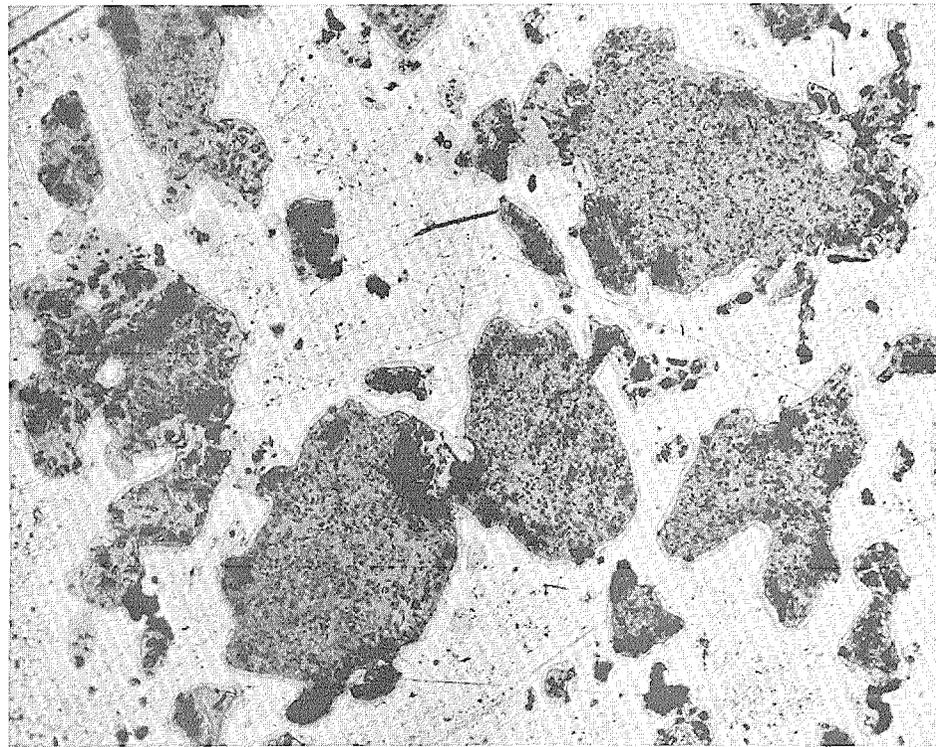
Fig. 3. Microstructure of  $U_3SiAl$  Plates from Module-3
