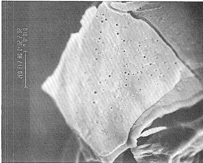
Fig. 5. Scanning Electron Micrograph of Fractured  $U_3SiAl$  Fuel Particle from Module-3 Plate
