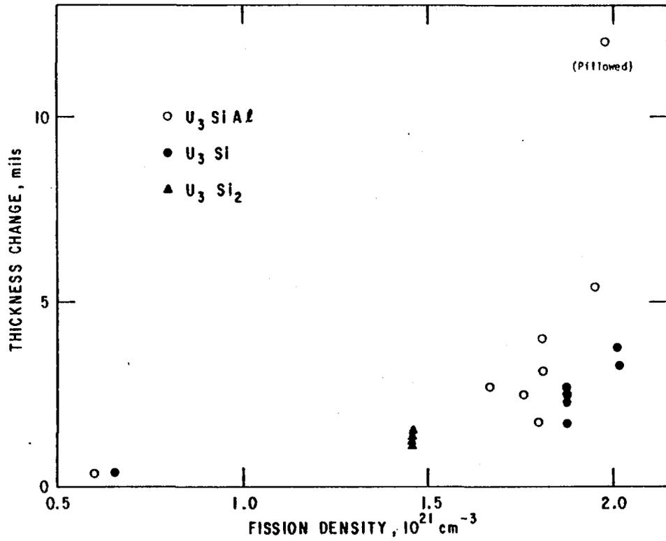
Fig. 1. Measured Increase in Fuel-plate Thickness.
