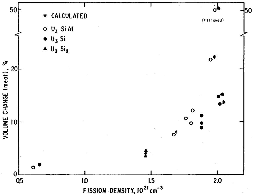
Fig. 2. Measured and Calculated Heat Volume Increase.
