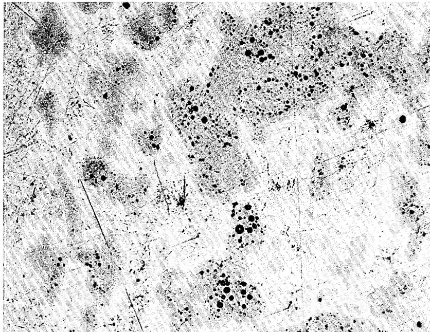
Fig. 7. Microstructure of U<sub>3</sub>Si Plate From Module 7; 200x
