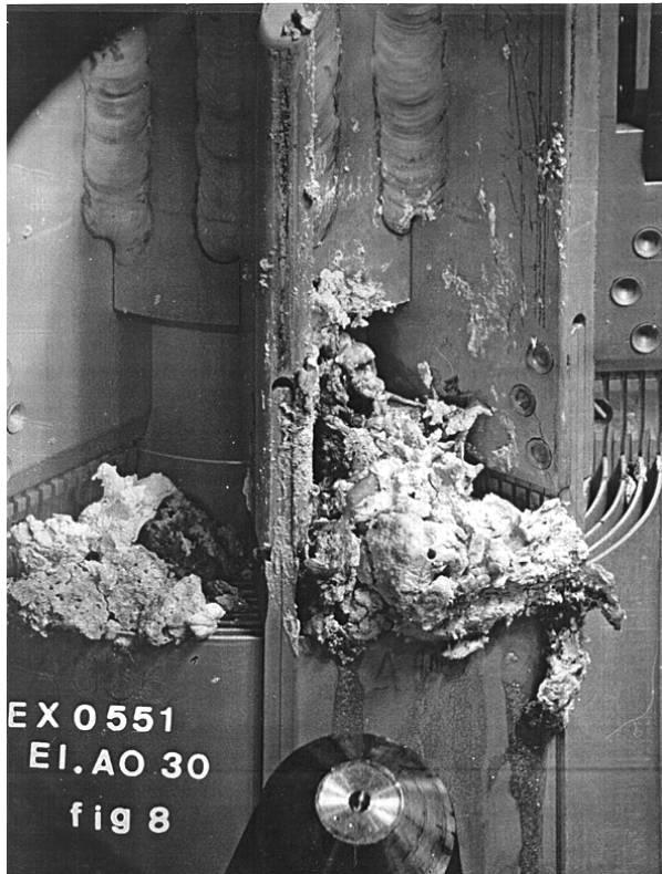
Figure 12: The damaged fuel element
