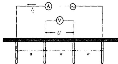
Figure 1. Disposition of the equipment of the measuring system according the Wenner's method
