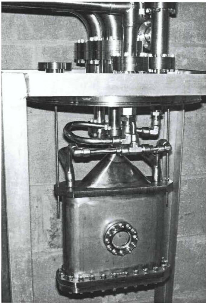
Figure 6. The 1.5 liter Amock moderator@ assembly (with the vacuum jacket removed).
