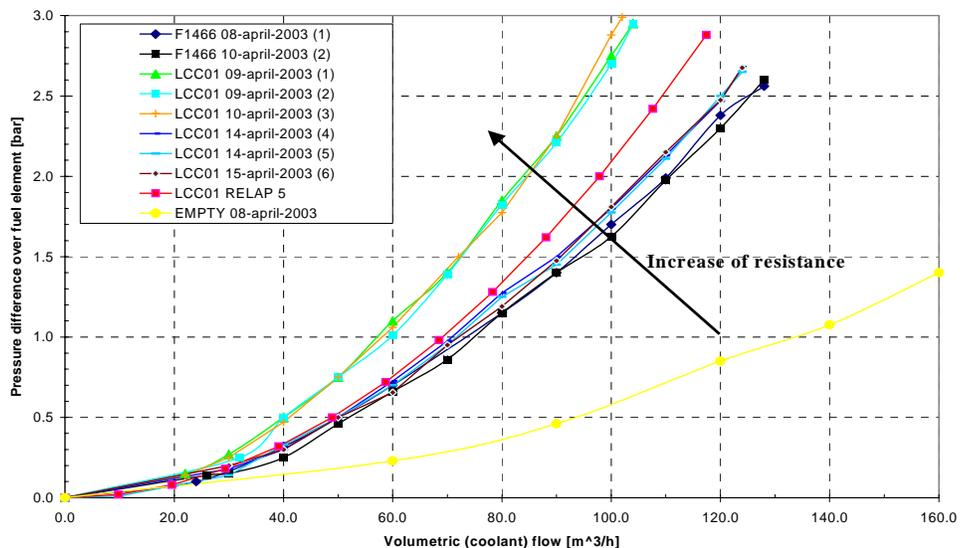
**Fig. 5. Hydraulic Test data.**
