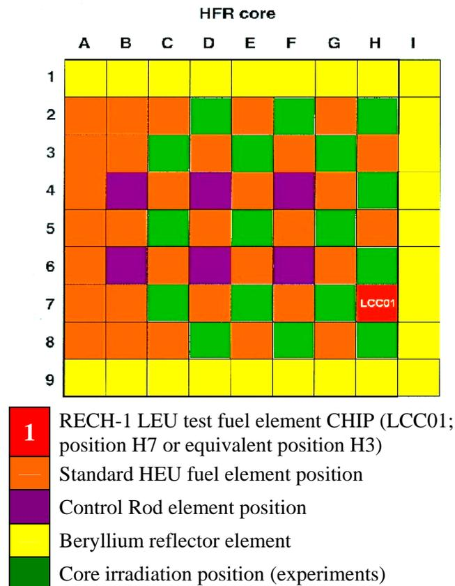
**Fig. 3. HFR core irradiation positions including RECH-1 test fuel element (H7 or H3 equivalent position)**
