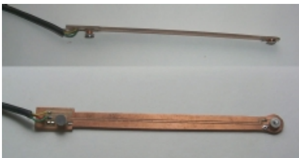
Figure 12 – Probe developed for MTR type fuel elements
