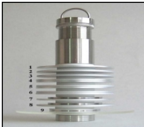
Figure 8 - Test rack used in the corrosion program.
