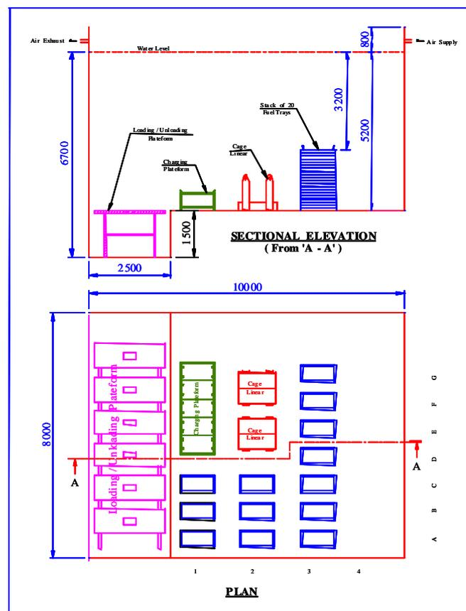
Fig. 2. Schematic Diagram of a typical spent fuel pool
