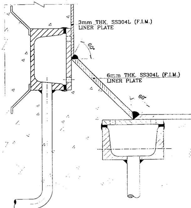
Fig. 5. Leak detection system
