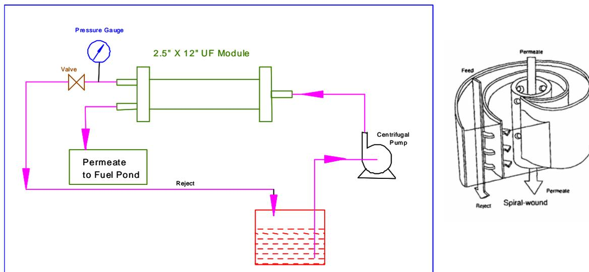
Fig. 7. UF module and the Schematic of the UF process
