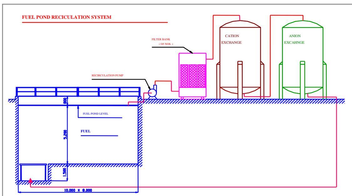
Fig. 6. Schematic diagram of the water polishing system
