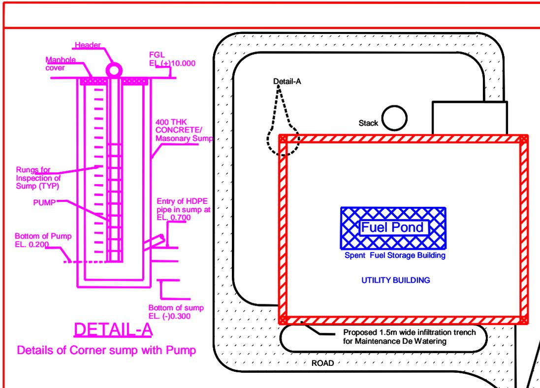
Fig. 4 Schematic diagram of the SFSF layout
