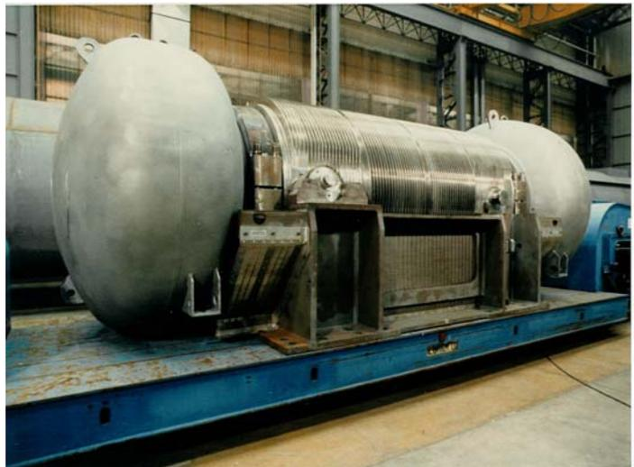
Fig. 4: AGN-1 cask with shock absorber.
