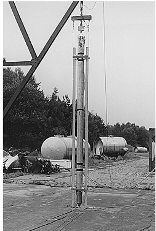
Figure 1. ESBB cask for the 9 m vertical drop test onto the bottom side shock absorber
