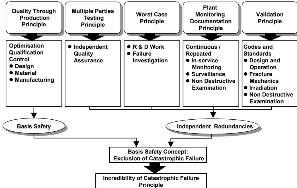
Figure 1: German Basis Safety Concept (BSC) schematically
