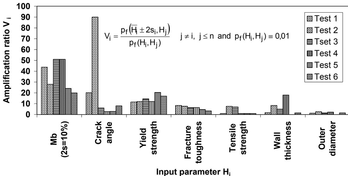
Figure 3: Influence on moment of crack initiation of piping components if the specific input parameter  $H_i$  deviates by  $2s_i$  from its mean value
