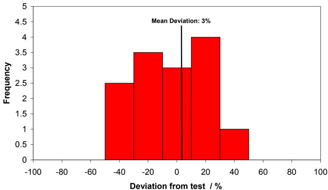
Figure 2: Comparison of moment for crack initiation calculated by the R6-Method with the experimental results of the tests (15 pipe component tests)
