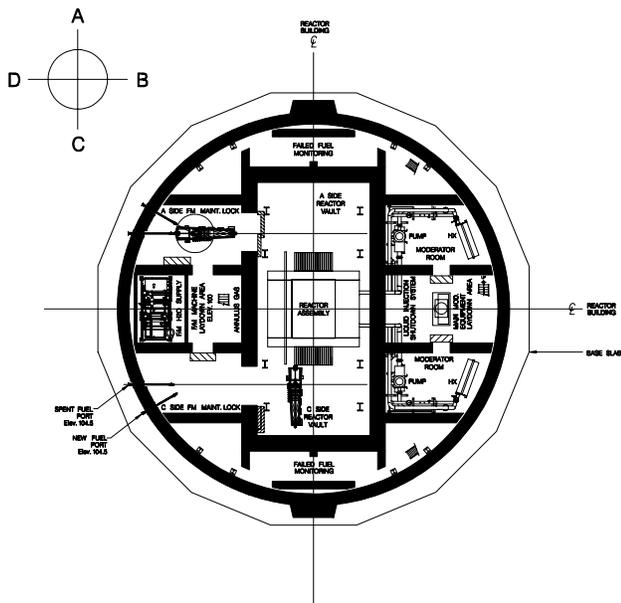
Figure 2 – Plan View of Reactor Building
