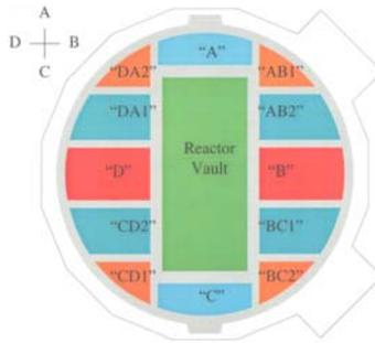
**Figure 4 – Plan View of Reactor Building Vertical Installation Compartments**
