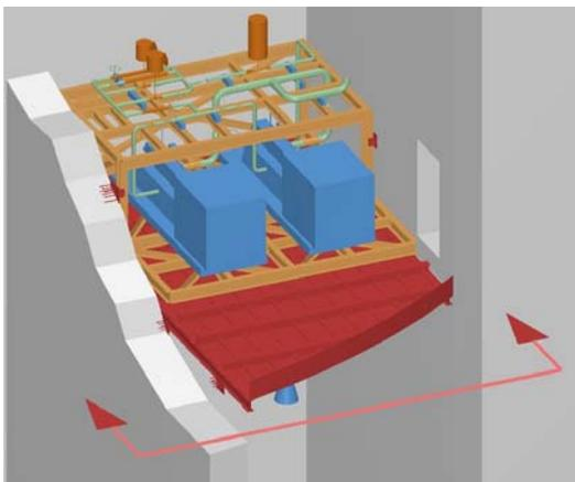
**Figure 7 – Example of a Module Supported from Internal Structure (Requiring Concrete in Base) (see Figure 10 for installation sequence)**
