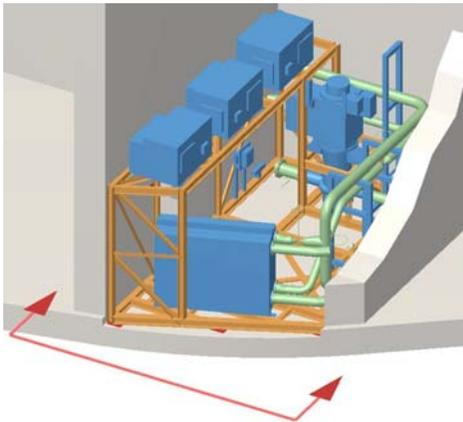
**Figure 5 – Example of a Module on the Base Slab (see Figure 8 for installation sequence)**
