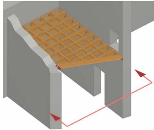
**Figure 6 – Example of a Module Supported from Internal Structure (Not Requiring Concrete in Base) (see Figure 9 for installation sequence)**
