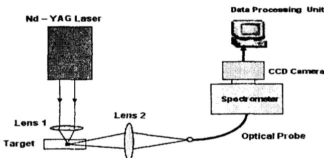
Fig.(1) LIBS Experimental Setup
