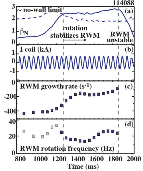
Fig. 4. (a)  $\beta_N$  is increased above the no-wall limit. (b) The I coil generates a rotating  $n = 1$  field with  $\omega_{\text{ext}}/(2\pi) = 20$  Hz. (c) RWM growth rate and (d) mode rotation frequency are obtained from the RFA measured at  $\omega_{\text{ext}}$  with midplane saddle loops, Eq. (8).
