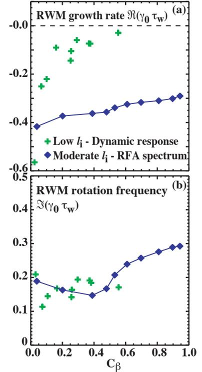
Fig. 6. RWM growth rate (a) and mode rotation frequency (b) obtained from the dynamic response to C coil pulses in low- $l_i$  plasmas (crosses) and the RFA spectrum using rotating I coil fields in moderate- $l_i$  plasmas (diamonds).
