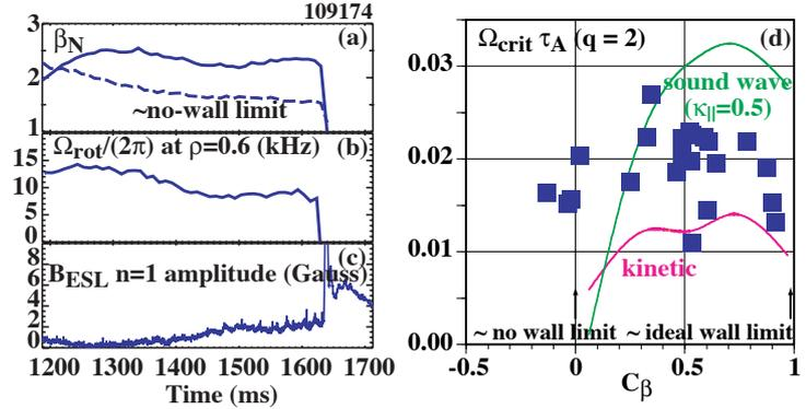
Fig. 5. (a) When  $\beta_N$  exceeds the no-wall limit, (b) the toroidal plasma rotation decreases until the onset of an  $n = 1$  RWM (c) seen with saddle loops in the midplane. (d) Measurements of  $\Omega_{\text{crit}} \tau_A$  at  $q = 2$  are compared with MARS predictions for sound wave damping ( $\kappa_{\parallel} = 0.5$ ) and kinetic damping.
