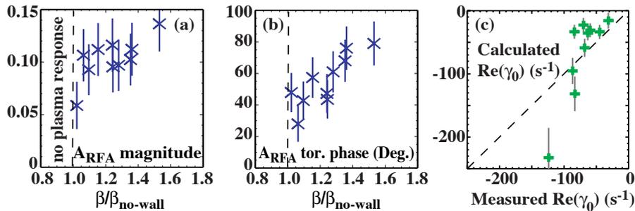
Fig. 2. RFA magnitude (a) and toroidal phase (b) for  $n = 1$  pulses with the C coil yield a value of the (negative) RWM growth rate (c) which is compared to the measured decay rate after the pulse is switched off.
