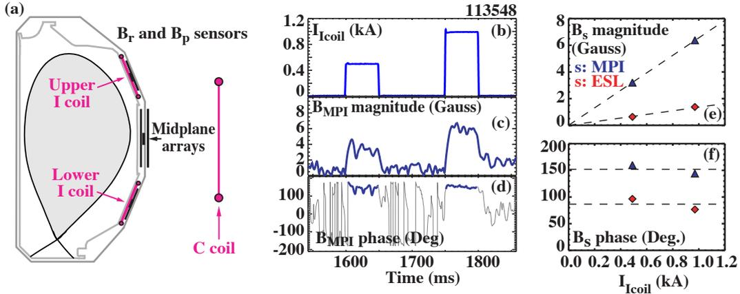
Fig. 1. (a) Poloidal cross-section of DIII-D plasma with the location of I and C coils and various magnetic sensors. (b) Resonant  $n = 1$  I coil pulses, (c) magnitude and (d) toroidal phase of the resulting  $n = 1$  plasma response measured with poloidal field probes on the midplane (MPI). (e) The magnitude of the plasma response measured with MPI sensors and saddle loops on the midplane (ESL) increases linearly with the applied current while (f) its toroidal phase remains constant.
