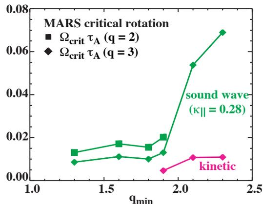
Fig. 9. MARS calculations of  $\Omega_{\text{crit}}\tau_A$  at the  $q = 2$  and  $q = 3$  surface in an DIII-D advanced tokamak scenario depend on  $q_{\text{min}}$ . Sound wave damping ( $\kappa_{\parallel} = 0.28$ ) and kinetic damping predict a significant increase of  $\Omega_{\text{crit}}\tau_A$  when  $q_{\text{min}}$  is raised above 2.
