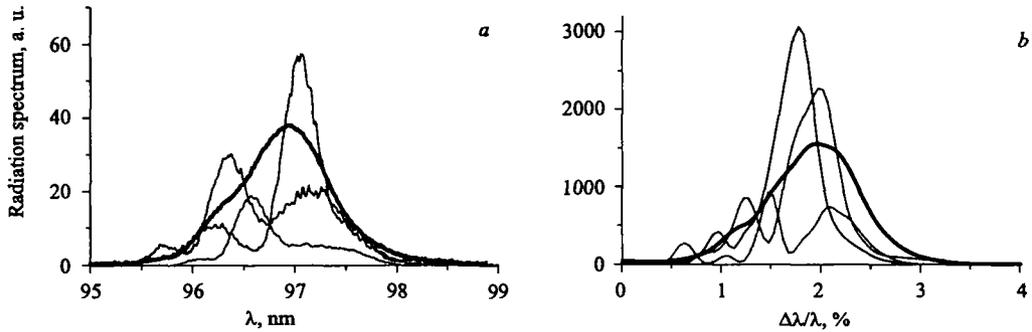
Fig. 4. Single-shot spectra (thin lines) and averaged spectrum (bold lines) of TTF FEL operating in the nonlinear regime: *a*) experimental data [1]; *b*) results of simulations with the code FAST
