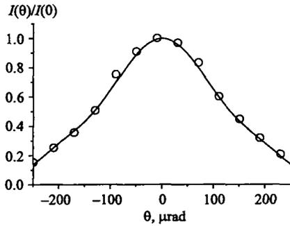
Fig. 5. Angular distribution of the radiation intensity in the far zone. TTF FEL operates in the nonlinear regime. Circles are experimental data [1], and curves represent results of simulations with the code FAST
