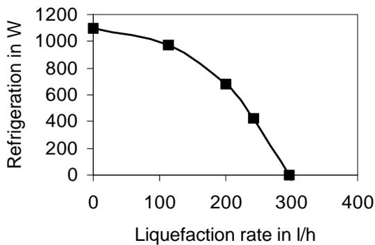
FIG. 6. Liquefaction Vs Refrigeration capacity of the Plant
