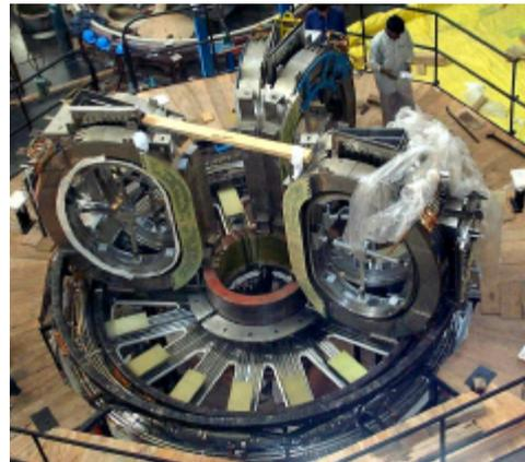
*FIG. 4. TF modules on support structure*
