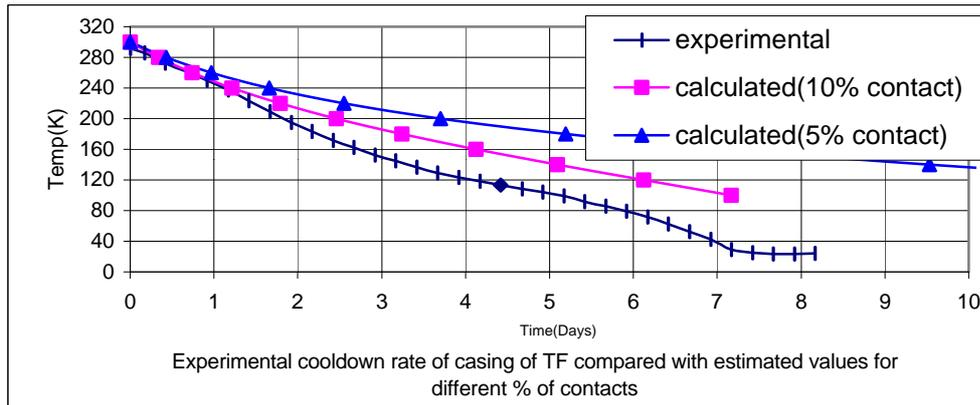
FIG. 11. Rate of cool down of the TF coils (experimental observations and theoretical estimates)
