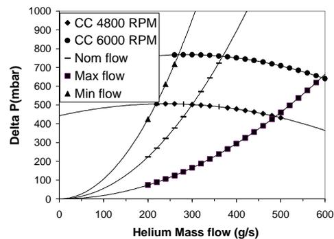
FIG. 7. Characteristics of cold circulator for the different speeds from test data
