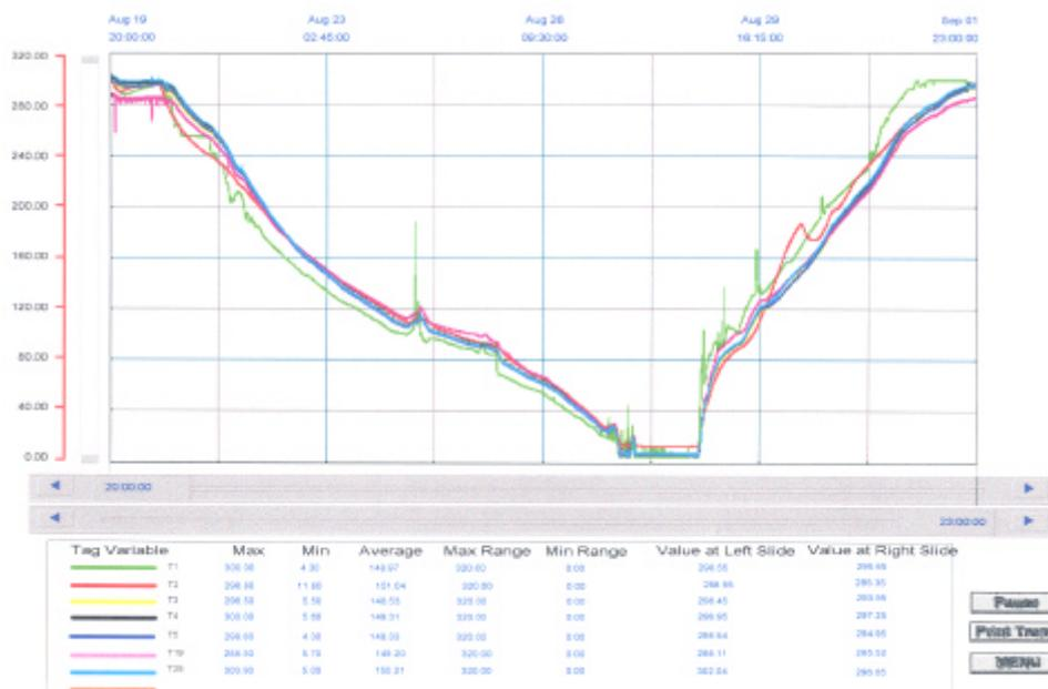
FIG.10. Cool down and warm up curves for the single TF coil
