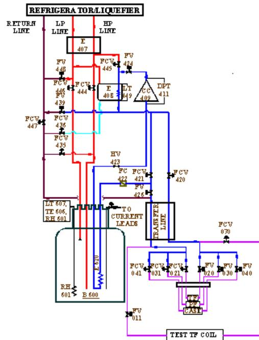
FIG.2. The schematics of the Helium Refrigerator/Liquefier with the integrated flow distribution system.
