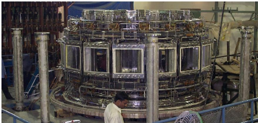
*FIG. 5. A view of complete assembly of the SCMS, vacuum vessel and LN<sub>2</sub> panels*
