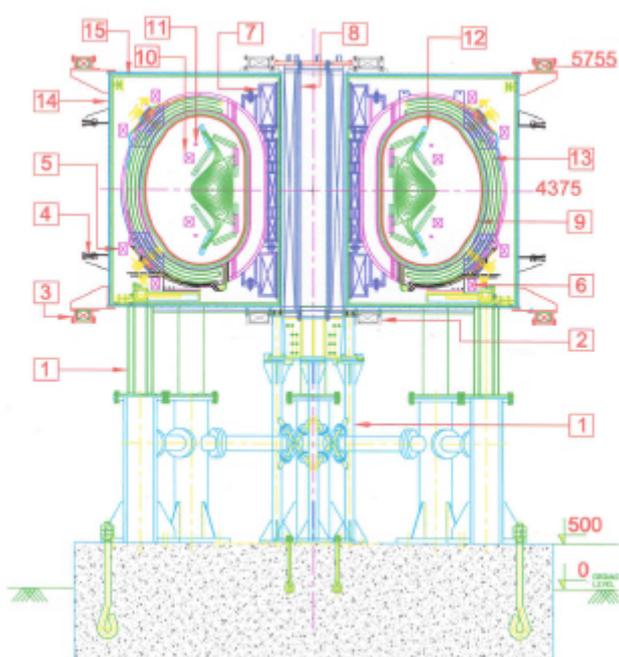
FIG.1 A cross-section of the SST-1 tokamak. (1 -Support Structure; 2-TR2 Coil ; 3-VF Coil; 4 -TR3 Coil; 5-PF5 Coil; 6-PF4 Coil; 7 -PF1, PF2 & PF3 Coils; 8-TR1 Coil; 9-Vacuum Vessel; 10 -PF6 Coil; 11-Feedback Coil; 12-PFC; 13 -TF Coil;14- Cryostat; 15- LN2 Panels)
