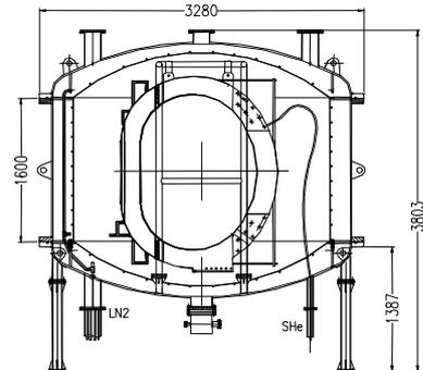
FIG. 8. Schematic diagram of the test set up for TF coil cool down.
