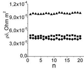
FIG. 3. Dependence  $\rho_i \delta_i$  of thermocycle number ( $n$ ) 20°C per sec
