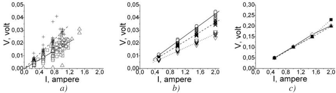
FIG. 1. Voltage-current characteristic of insulating coatings
