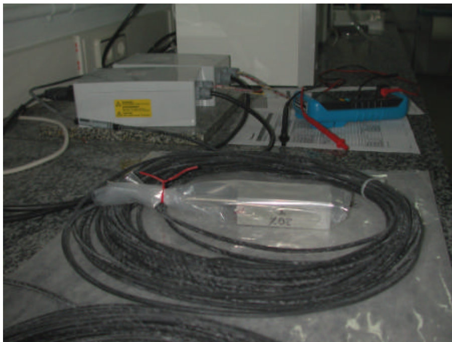
Figure 4: Measurement of the relative humidity inside a block of bentonite
