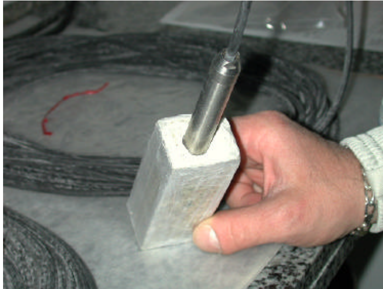
Figure 3: Bentonite compacted block with a hole drilled for the insertion of the RH sensor
