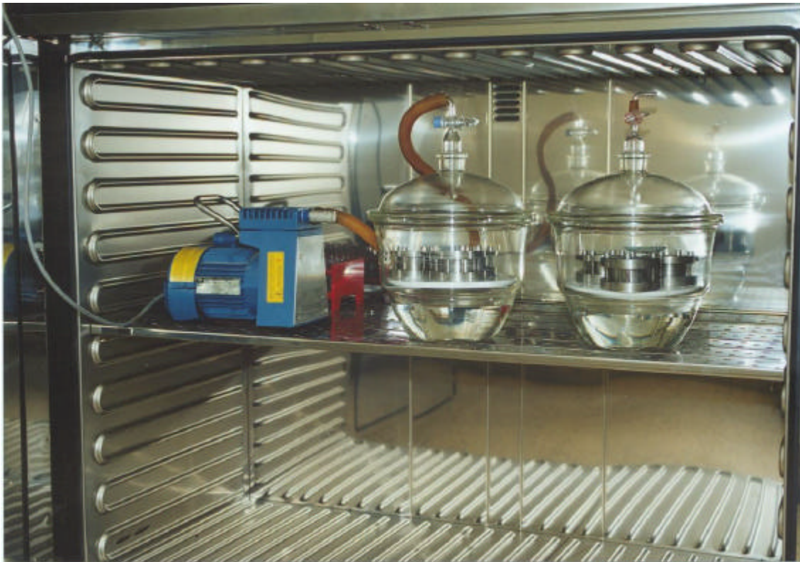
Figure 12: Desiccators with non-deformable cells inside the oven at the moment of vacuum generation
