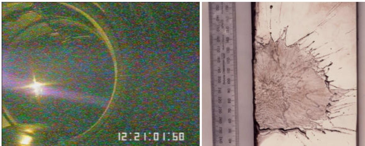
*Fig. 1 : Left : Runaway Electron Impact on the Outboard Limiter of Tore Supra
