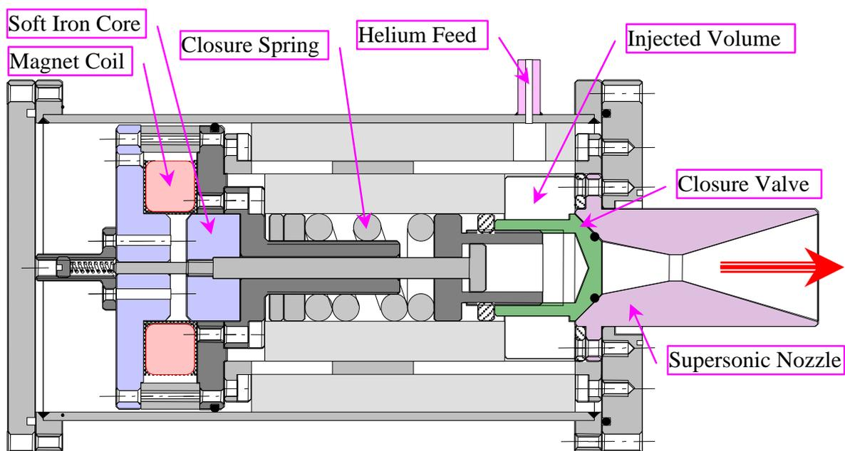
Fig 2. Tore Supra Massive Gas Injector
