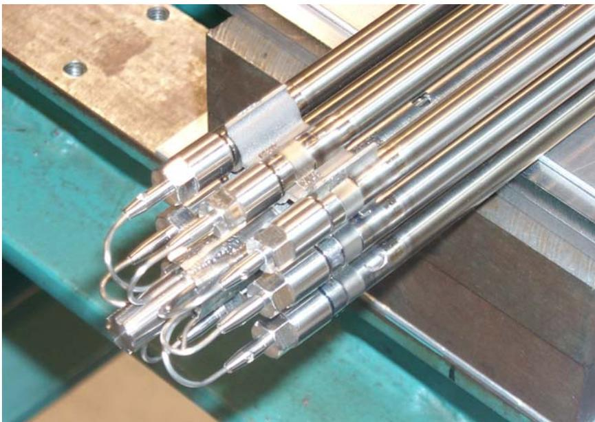
*Bottom of the OMICO instrumented fuel bundle. All pins are equipped with a central high temperature thermocouple connected via the lower end plug and a pressure transducer connected via the upper end plug*
