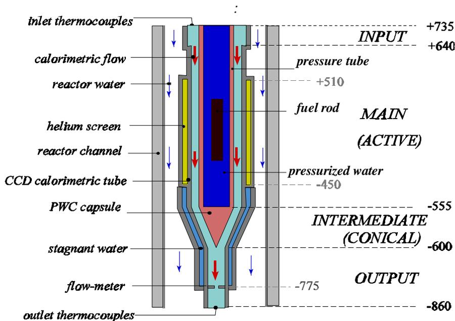
*Power Ramping - Scheme of the PWC/CCD device (Pressurized Water Capsule/ Calibration and Cycling Device) with axial reactor coordinates in mm ('0' being the centre of the 76 mm high BR2 core).*
