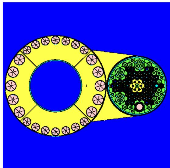
*The right this figure shows the modelling of a carousel-type rotating irradiation facility located in the reactor pool outside of the BR2 vessel for Si-doping production activities.*
