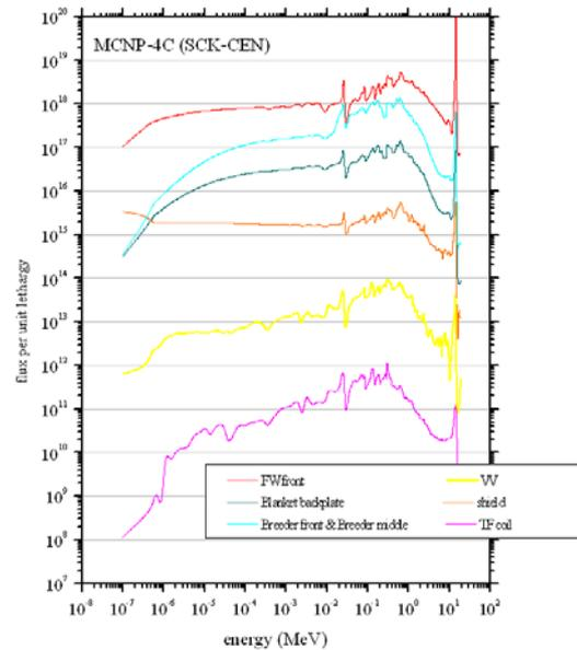
On the right the calculated neutron spectra in different parts of the tokamak of ITER
