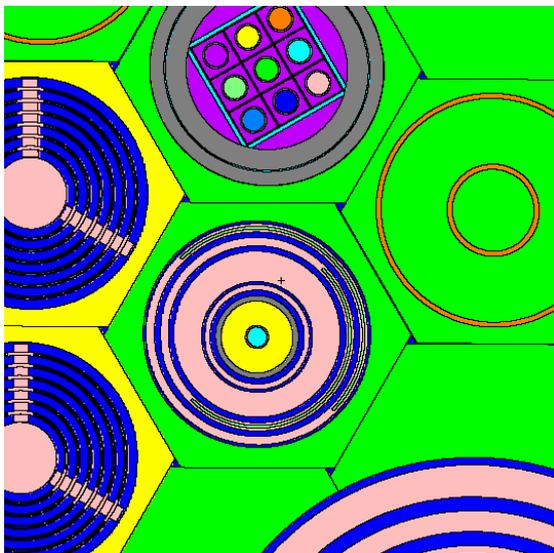
*Modelling of newly proposed irradiation devices: this figure illustrates the modelling of a proposed device for power ramping on single fuel pins using various rotating absorber screens. The figure gives a cross section of the BR2 core at +30 cm above the mid-plane.*
