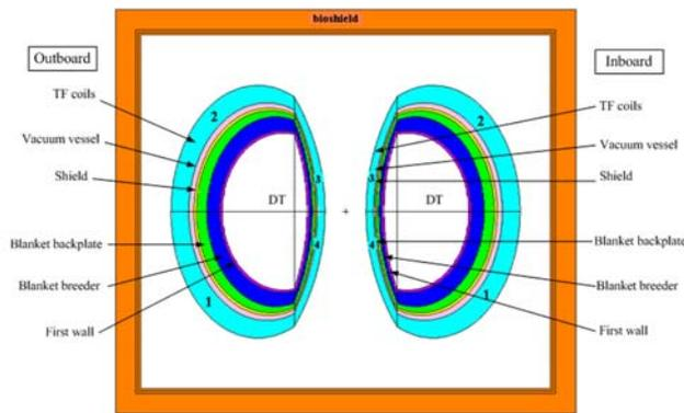
On the left the MCNP calculation model of the tokamak building of ITER. This model has been used for the evaluation of the activation of the biological shield.
