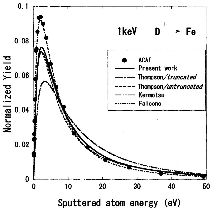
Fig.3 Normalized yields of atoms sputtered from a Fe material irradiated by 1 keV D<sup>+</sup> ions at normal incidence vs. sputtered atom energy in eV. Refer to Fig. 1 for legend.
