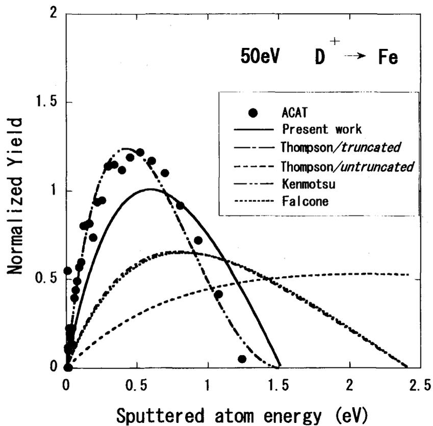
Fig.1 Normalized yields of atoms sputtered from a Fe material irradiated by 50 eV  $D^+$  ions at normal incidence vs. sputtered atom energy in eV. The legend shows the curves obtained with the different formulas. The closed circles are the data calculated with the ACAT code. Note that the *truncated* Thompson and the Falcone curves completely overlap.
