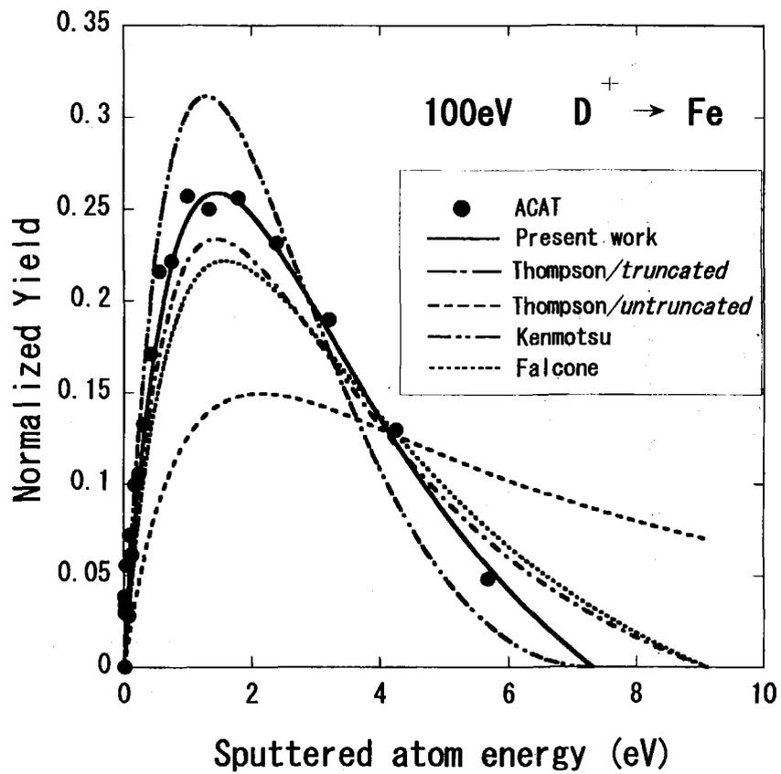
Fig.2 Normalized yields of atoms sputtered from a Fe material irradiated by 100 eV D<sup>+</sup> ions at normal incidence vs. sputtered atom energy in eV. Refer to Fig. 1 for legend.
