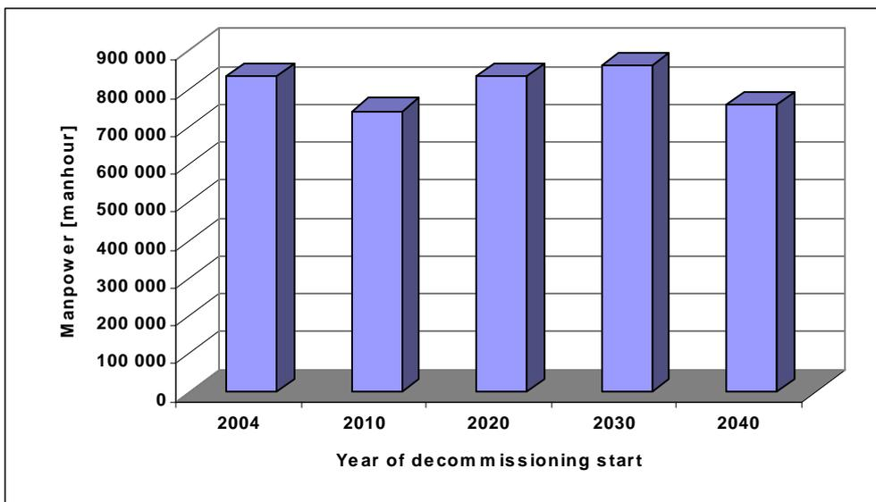
**Figure 32:** Manpower for different calculated options. These options differ in decommissioning start time (2004, 2010, 2020, 2030 and 2040) for decommissioning scenario S1. Typical radionuclide composition and the level of contamination of non-accident NPP V-2. Applied pre-dismantling decontamination.
