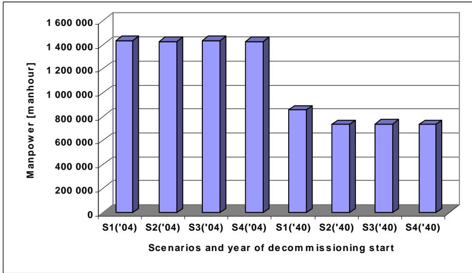
**Figure 14:** Manpower for different calculated options. These options differ in decommissioning scenarios (from S1 to S4) and decommissioning start time (either 2004 or 2040). Typical radionuclide composition for NPP A-1. No pre-dismantling decontamination applied.
