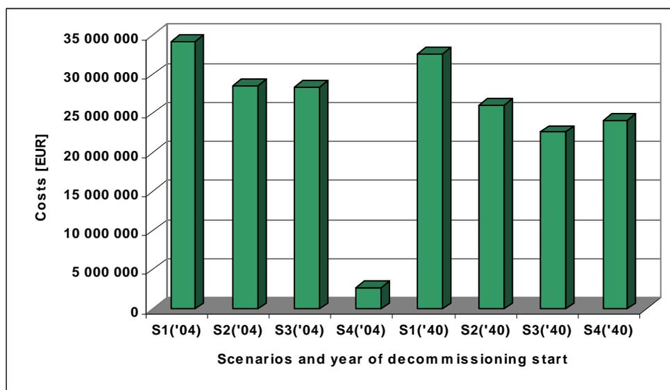
**Figure 22:** Costs for different calculated options. These options differ in decommissioning scenarios (from S1 to S4) and decommissioning start time (either 2004 or 2040). Typical radionuclide composition for NPP A-1 with 10-times lower contamination level. Applied pre-dismantling decontamination.
