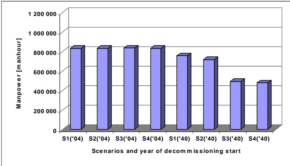
**Figure 26:** Manpower for different calculated options. These options differ in decommissioning scenarios (from S1 to S4) and decommissioning start time (either 2004 or 2040). Typical radionuclide composition and the level of contamination of non-accident NPP V-2. Applied pre-dismantling decontamination.
