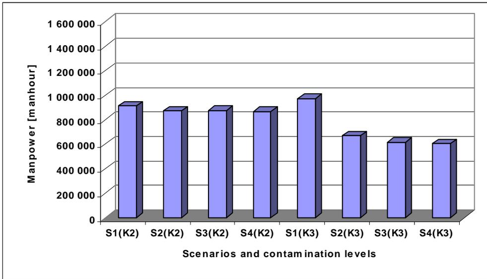
**Figure 11:** Manpower for different calculated options. These options differ in decommissioning scenarios (from S1 to S4) and level of contamination of decommissioned technology equipment (either K2 or K3 level with typical radionuclide composition for NPP A-1). Applied pre-dismantling decontamination.
