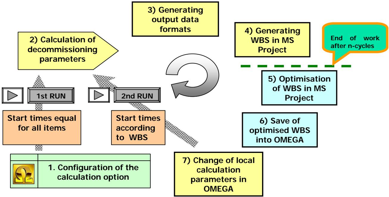
Figure 1: Schematic set of OMEGA code operations
