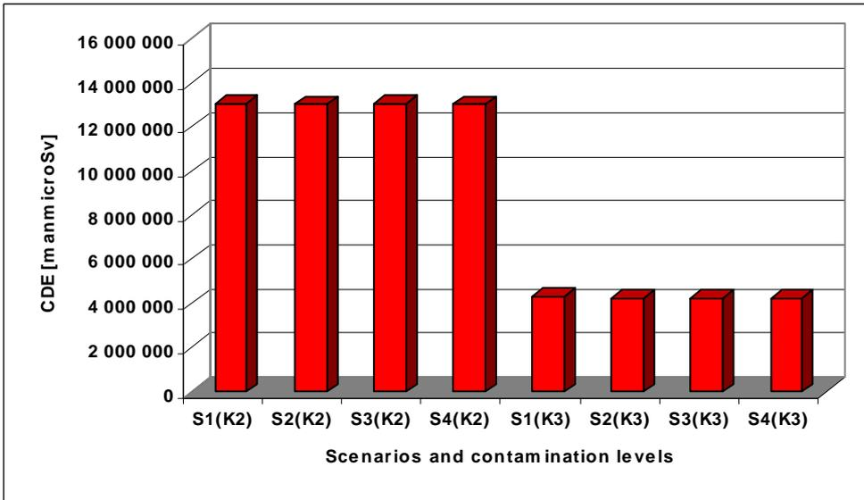
**Figure 9:** Collective dose equivalent for different calculated options. These options differ in decommissioning scenarios (from S1 to S4) and level of contamination of decommissioned technology equipment (either K2 or K3 level with typical radionuclide composition for NPP A-1). No pre-dismantling decontamination applied.
