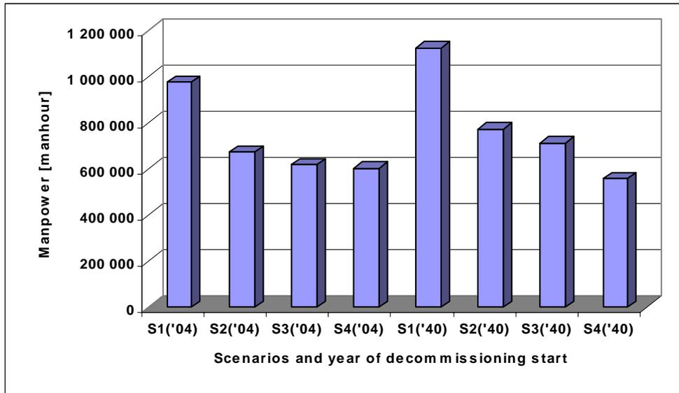
**Figure 20:** Manpower for different calculated options. These options differ in decommissioning scenarios (from S1 to S4) and decommissioning start time (either 2004 or 2040). Typical radionuclide composition for NPP A-1 with 10-times lower contamination level. Applied pre-dismantling decontamination.
