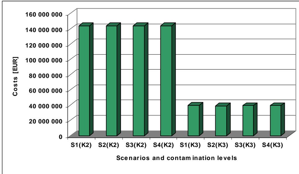
**Figure 10:** Costs for different calculated options. These options differ in decommissioning scenarios (from S1 to S4) and level of contamination of decommissioned technology equipment (either K2 or K3 level with typical radionuclide composition for NPP A-1). No pre-dismantling decontamination applied.
