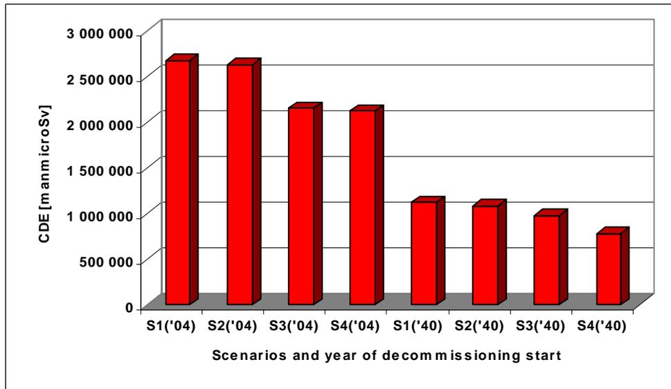
**Figure 30:** Collective dose equivalent for different calculated options. These options differ in decommissioning scenarios (from S1 to S4) and decommissioning start time (either 2004 or 2040). Typical radionuclide composition for non-accident NPP V-2 with 10-times lower contamination level. Applied pre-dismantling decontamination.
