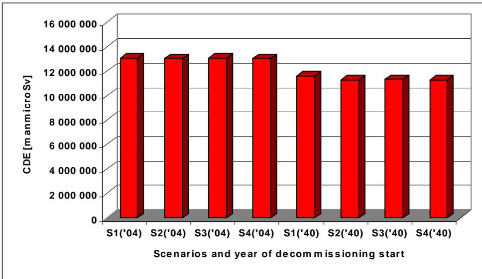
**Figure 15:** Collective dose equivalent for different calculated options. These options differ in decommissioning scenarios (from S1 to S4) and decommissioning start time (either 2004 or 2040). Typical radionuclide composition for NPP A-1. No pre-dismantling decontamination applied.
