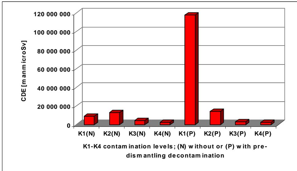
**Figure 6:** Collective dose equivalent for different calculated options. These options differ in level of contamination of decommissioned technology equipment (with typical radionuclide composition for NPP A-1, decommissioning scenario S1) without (N) or with (P) pre-dismantling decontamination.
