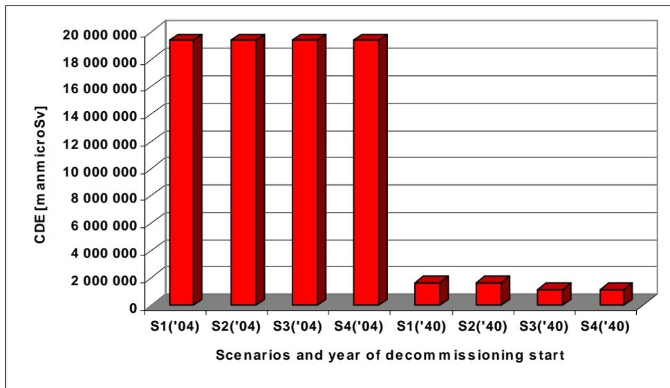
**Figure 24:** Collective dose equivalent for different calculated options. These options differ in decommissioning scenarios (from S1 to S4) and decommissioning start time (either 2004 or 2040). Typical radionuclide composition and the level of contamination of non-accident NPP V-2. No pre-dismantling decontamination applied.
