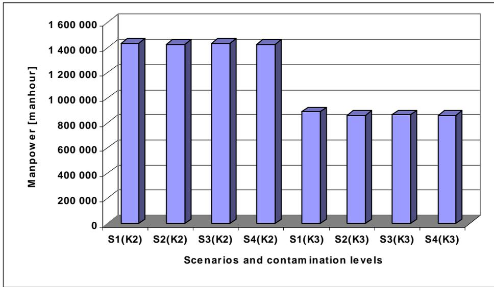
**Figure 8:** Manpower for different calculated options. These options differ in decommissioning scenarios (from S1 to S4) and level of contamination of decommissioned technology equipment (either K2 or K3 level with typical radionuclide composition for NPP A-1). No pre-dismantling decontamination applied.
