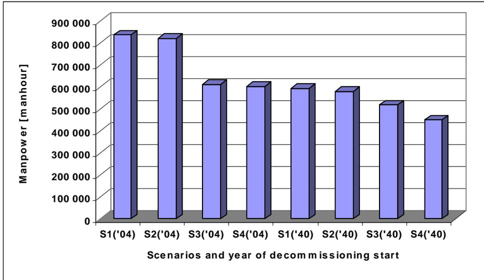
**Figure 29:** Manpower for different calculated options. These options differ in decommissioning scenarios (from S1 to S4) and decommissioning start time (either 2004 or 2040). Typical radionuclide composition for non-accident NPP V-2 with 10-times lower contamination level. Applied pre-dismantling decontamination.
