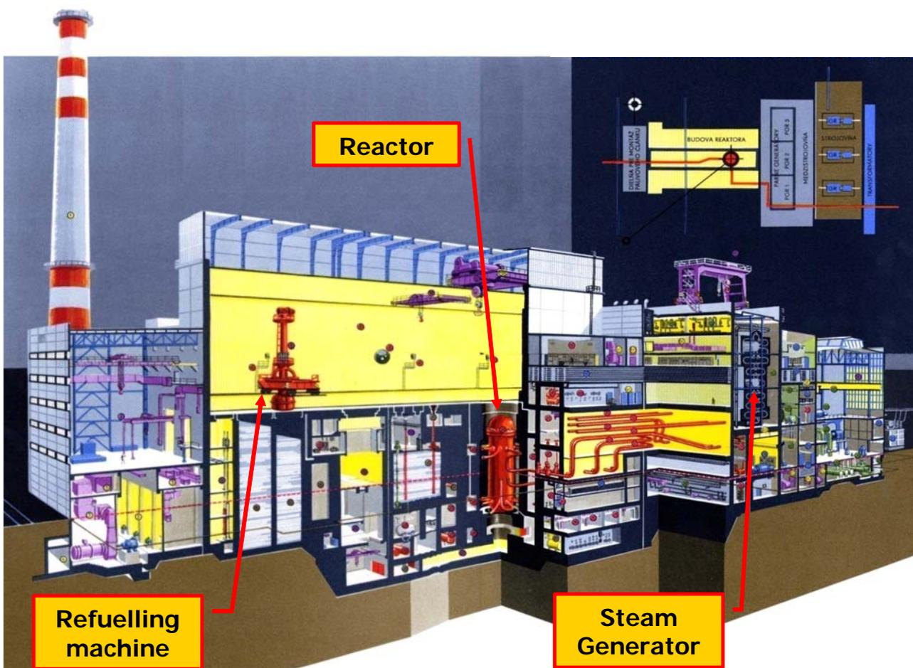
**Figure 2:** A-1 NPP main operation building
