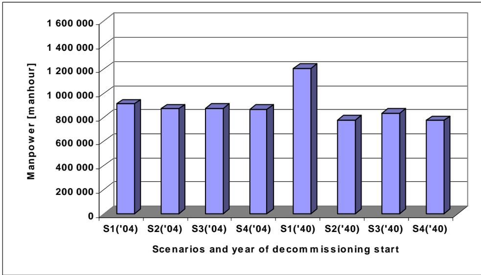
**Figure 17:** Manpower for different calculated options. These options differ in decommissioning scenarios (from S1 to S4) and decommissioning start time (either 2004 or 2040). Typical radionuclide composition for NPP A-1. Applied pre-dismantling decontamination.
