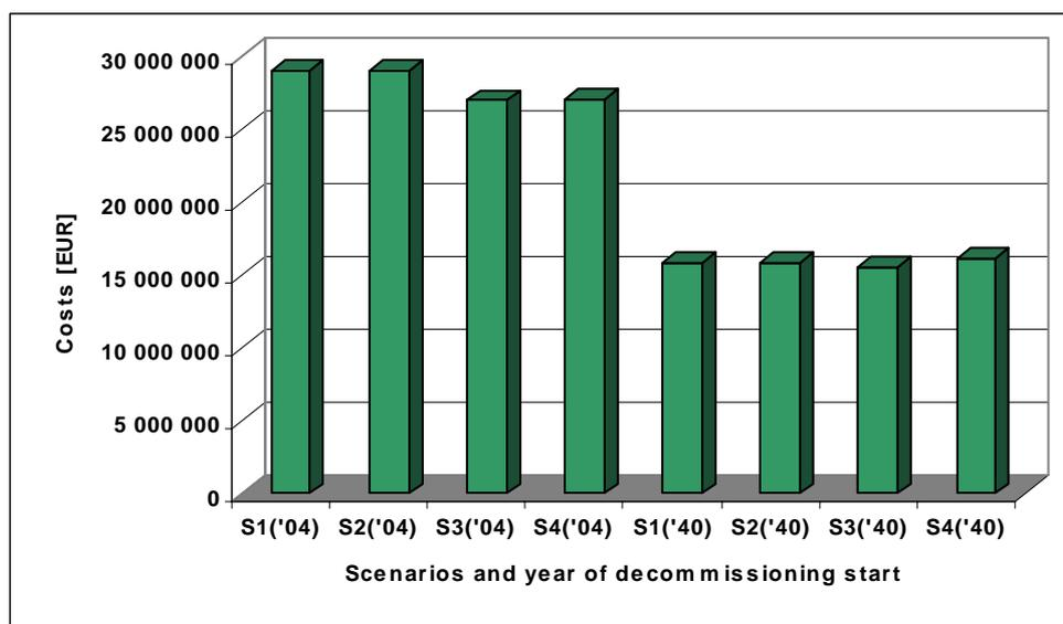
**Figure 31:** Costs for different calculated options. These options differ in decommissioning scenarios (from S1 to S4) and decommissioning start time (either 2004 or 2040). Typical radionuclide composition for non-accident NPP V-2 with 10-times lower contamination level. Applied pre-dismantling decontamination.
