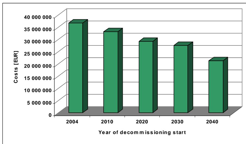
**Figure 34:** Costs for different calculated options. These options differ in decommissioning start time (2004, 2010, 2020, 2030 and 2040) for decommissioning scenario S1. Typical radionuclide composition and the level of contamination of non-accident NPP V-2. Applied pre-dismantling decontamination.
