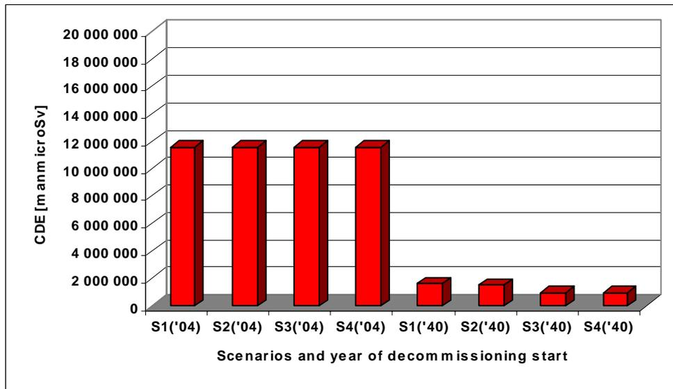
**Figure 27:** Collective dose equivalent for different calculated options. These options differ in decommissioning scenarios (from S1 to S4) and decommissioning start time (either 2004 or 2040). Typical radionuclide composition and the level of contamination of non-accident NPP V-2. Applied pre-dismantling decontamination.
