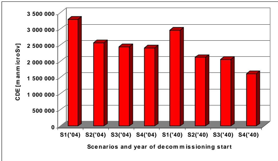
**Figure 21:** Collective dose equivalent for different calculated options. These options differ in decommissioning scenarios (from S1 to S4) and decommissioning start time (either 2004 or 2040). Typical radionuclide composition for NPP A-1 with 10-times lower contamination level. Applied pre-dismantling decontamination.
