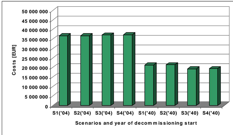
**Figure 28:** Costs for different calculated options. These options differ in decommissioning scenarios (from S1 to S4) and decommissioning start time (either 2004 or 2040). Typical radionuclide composition and the level of contamination of non-accident NPP V-2. Applied pre-dismantling decontamination.
