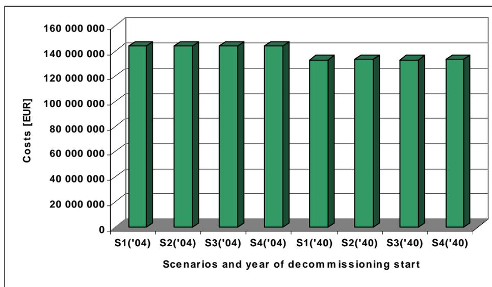
**Figure 16:** Costs for different calculated options. These options differ in decommissioning scenarios (from S1 to S4) and decommissioning start time (either 2004 or 2040). Typical radionuclide composition for NPP A-1. No pre-dismantling decontamination applied.
