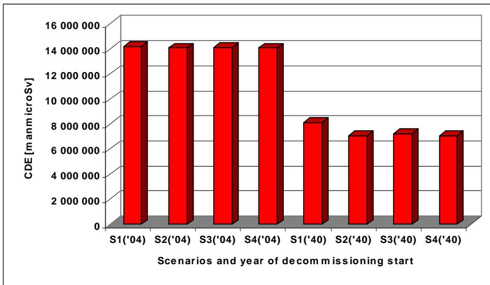
**Figure 18:** Collective dose equivalent for different calculated options. These options differ in decommissioning scenarios (from S1 to S4) and decommissioning start time (either 2004 or 2040). Typical radionuclide composition for NPP A-1. Applied pre-dismantling decontamination.
