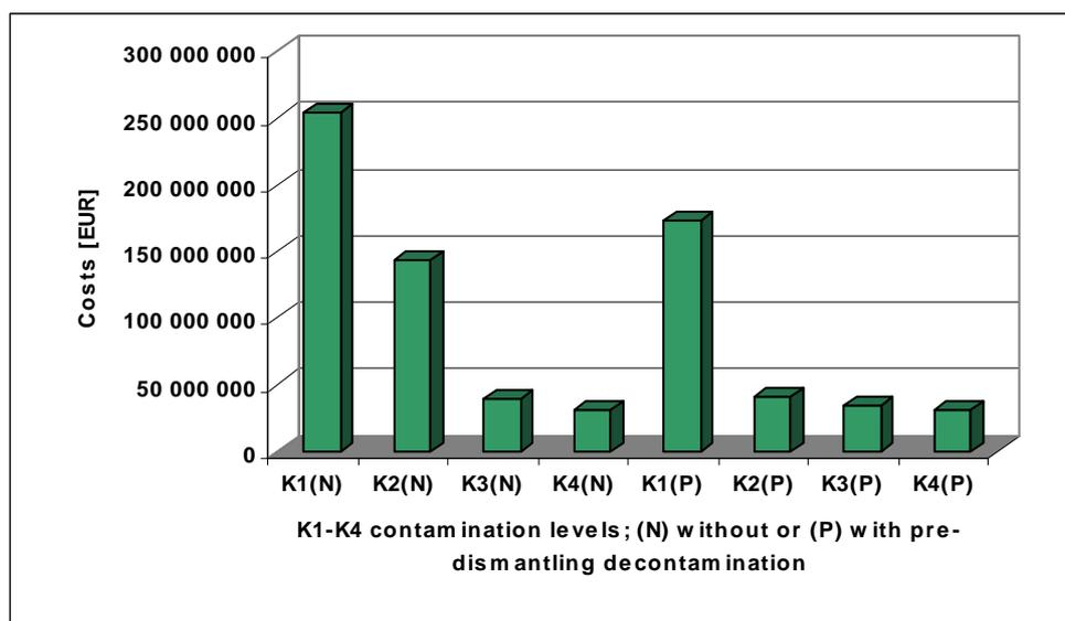
**Figure 7:** Costs for different calculated options. These options differ in level of contamination of decommissioned technology equipment (with typical radionuclide composition for NPP A-1, decommissioning scenario S1) without (N) or with (P) pre-dismantling decontamination.
