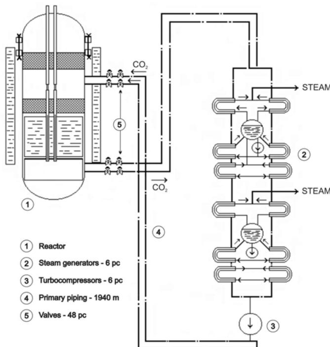
Contaminated parts of A-1 NPP primary circuit shown in **Figure 3** excluding reactor pressure vessel are subject to OMEGA code decommissioning cost calculation, that is introduced in the following chapters.
