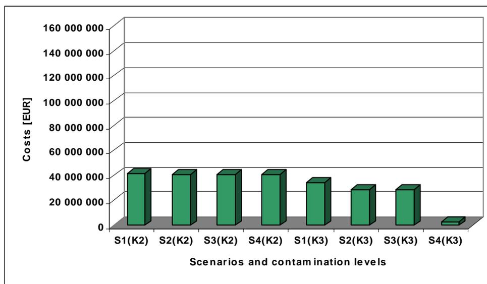
**Figure 13:** Costs for different calculated options. These options differ in decommissioning scenarios (from S1 to S4) and level of contamination of decommissioned technology equipment (either K2 or K3 level with typical radionuclide composition for NPP A-1). Applied pre-dismantling decontamination.
