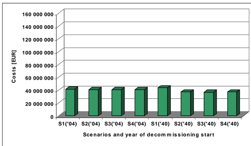
**Figure 19:** Costs for different calculated options. These options differ in decommissioning scenarios (from S1 to S4) and decommissioning start time (either 2004 or 2040). Typical radionuclide composition for NPP A-1. Applied pre-dismantling decontamination.
