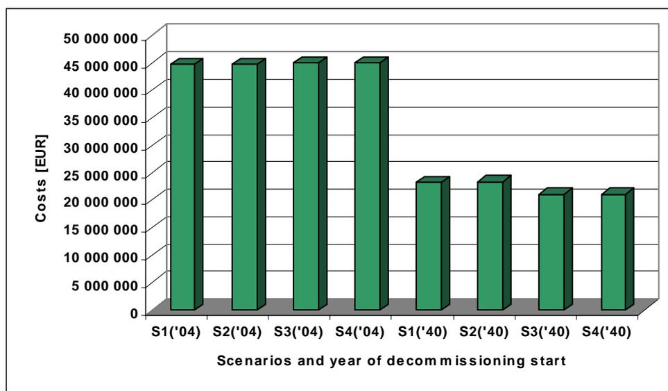
**Figure 25:** Costs for different calculated options. These options differ in decommissioning scenarios (from S1 to S4) and decommissioning start time (either 2004 or 2040). Typical radionuclide composition and the level of contamination of non-accident NPP V-2. No pre-dismantling decontamination applied.
