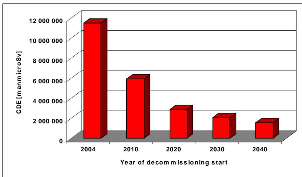
**Figure 33:** Collective dose equivalent for different calculated options. These options differ in decommissioning start time (2004, 2010, 2020, 2030 and 2040) for decommissioning scenario S1. Typical radionuclide composition and the level of contamination of non-accident NPP V-2. Applied pre-dismantling decontamination.
