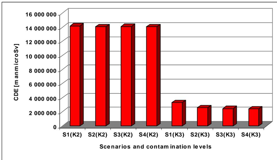
**Figure 12:** Collective dose equivalent distribution for different calculated options. These options differ in decommissioning scenarios (from S1 to S4) and level of contamination of decommissioned technology equipment (either K2 or K3 level with typical radionuclide composition for NPP A-1). Applied pre-dismantling decontamination.
