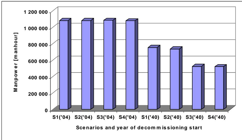
**Figure 23:** Manpower for different calculated options. These options differ in decommissioning scenarios (from S1 to S4) and decommissioning start time (either 2004 or 2040). Typical radionuclide composition and the level of contamination of non-accident NPP V-2. No pre-dismantling decontamination applied.
