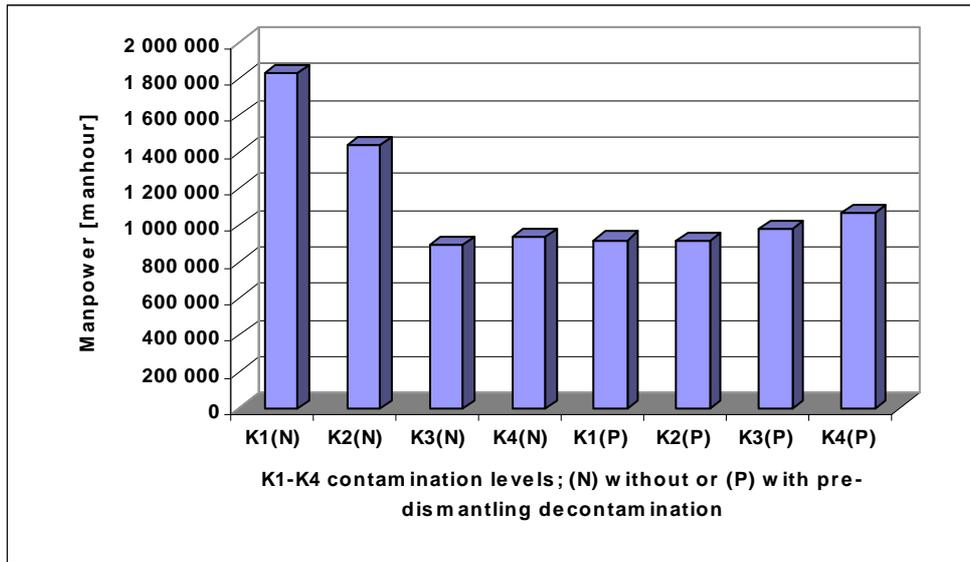
**Figure 5:** Manpower for different calculated options. These options differ in level of contamination of decommissioned technology equipment (with typical radionuclide composition for NPP A-1, decommissioning scenario S1) without (N) or with (P) pre-dismantling decontamination.
