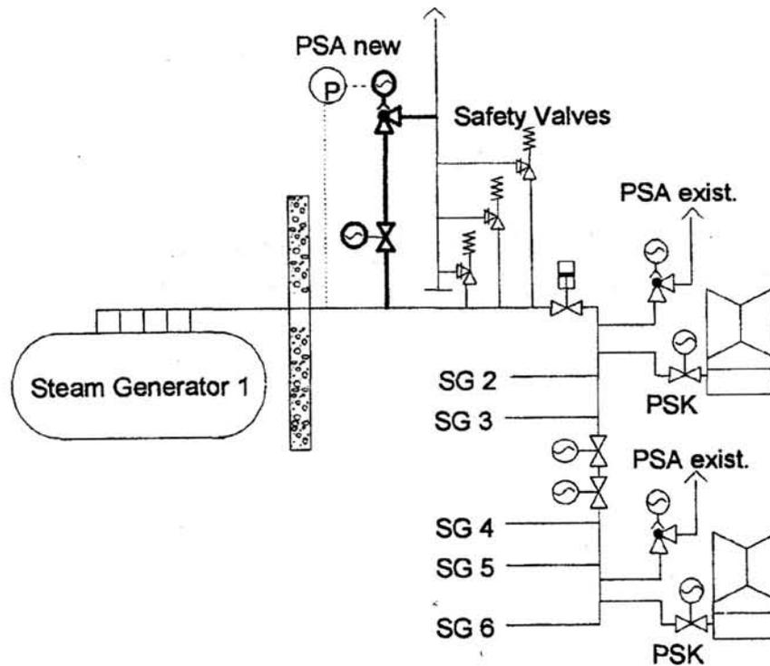
Fig. 2: Configuration of the Systems for Secondary Bleed
