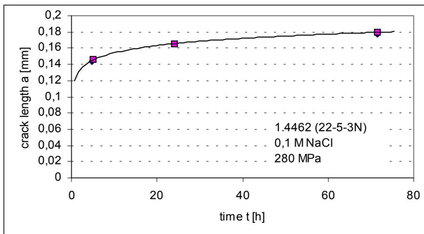
Figure 4. Dependence of crack length of time to fracture in 0,1 M NaCl
