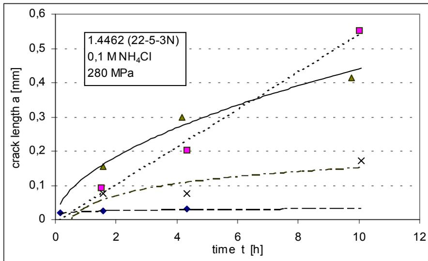
Figure 5. Dependence of crack length of time to fracture in 0,1 M NH<sub>4</sub>Cl.
