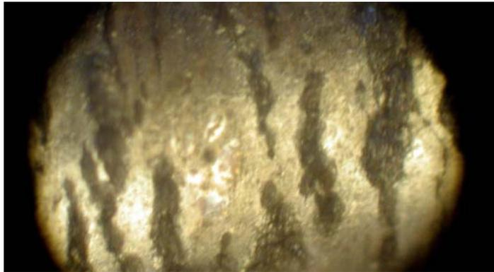
Figure 1 Monitoring of microcracks propagation “in situ” on the sample in the  $\text{NH}_4\text{Cl}$  solution (digital fotocamera, mag.  $\approx 80 \times$ )
