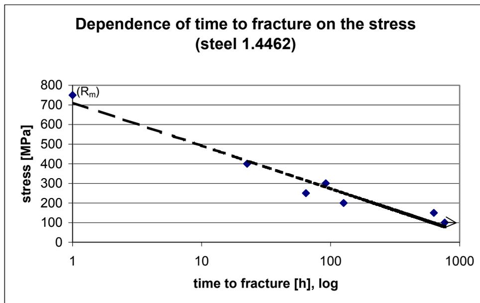
Figure 2. Dependence of time to fracture on applied stress. (0,1M NaCl)
