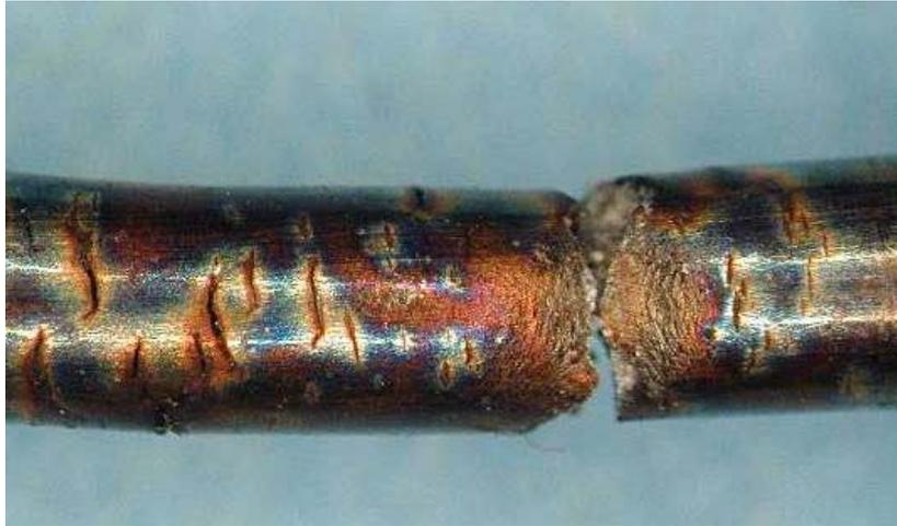
Figure 3. Typical corrosion cracks and fracture of tested material (NaCl) (stereomicroscopy 16x)
