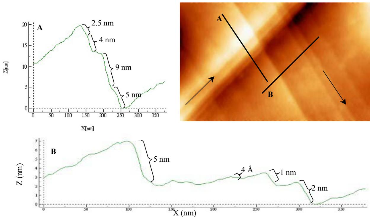
Fig. 4. Topographic contact AFM image of the surface inside a grain. The arrows indicate the trace of the slip planes: 2 different orientations. The profiles A and B taken along the lines A and B respectively show steps, which height can vary between 4 Å and 9 nm.
