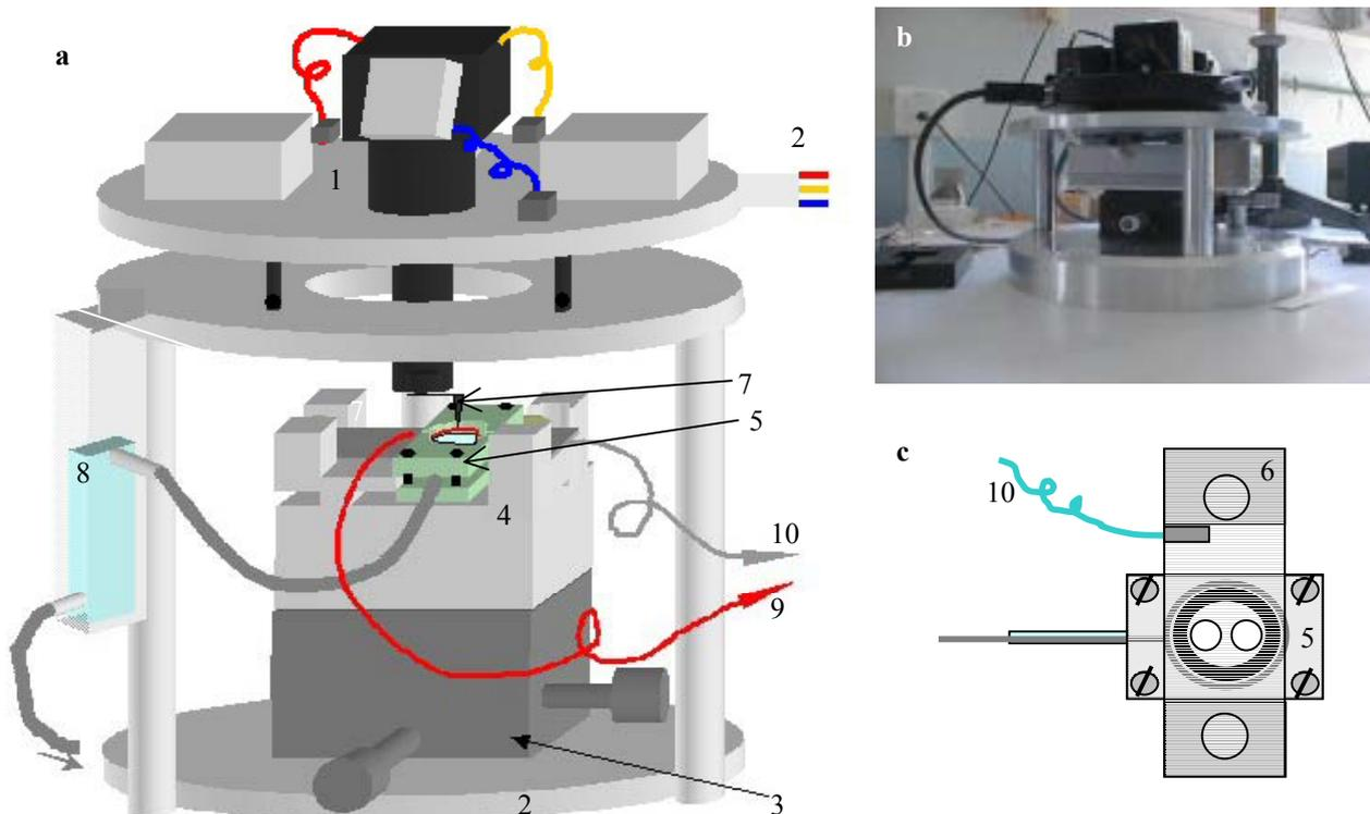
Fig. 2. a) general scheme of the set-up. 1, AFM head from Molecular Imaging in “stand-alone” configuration. 2, base isolated from high frequency vibrations. 3, X-Y vernier. 4, traction plate. 5, electrochemical cell. 6, sample. 7, AFM tip. 8, aqueous solution reservoir. 9, silver wire (CE). 10, copper wire connected to the test piece. b) picture of the experimental apparatus (scale 1:10). c) upper view of the electrochemical cell mounted on the sample.
