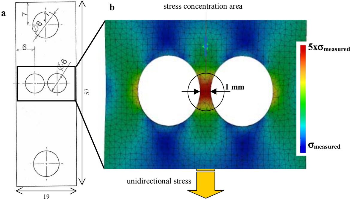
*Fig. 1. Test piece shape and dimensions (mm) (a), and strain simulation with CATIA V.5 (b). It shows the concentration of stress in a very small area for this conformation of the sample. The force applied is 350N. The figure shows the final state of the test piece.*
