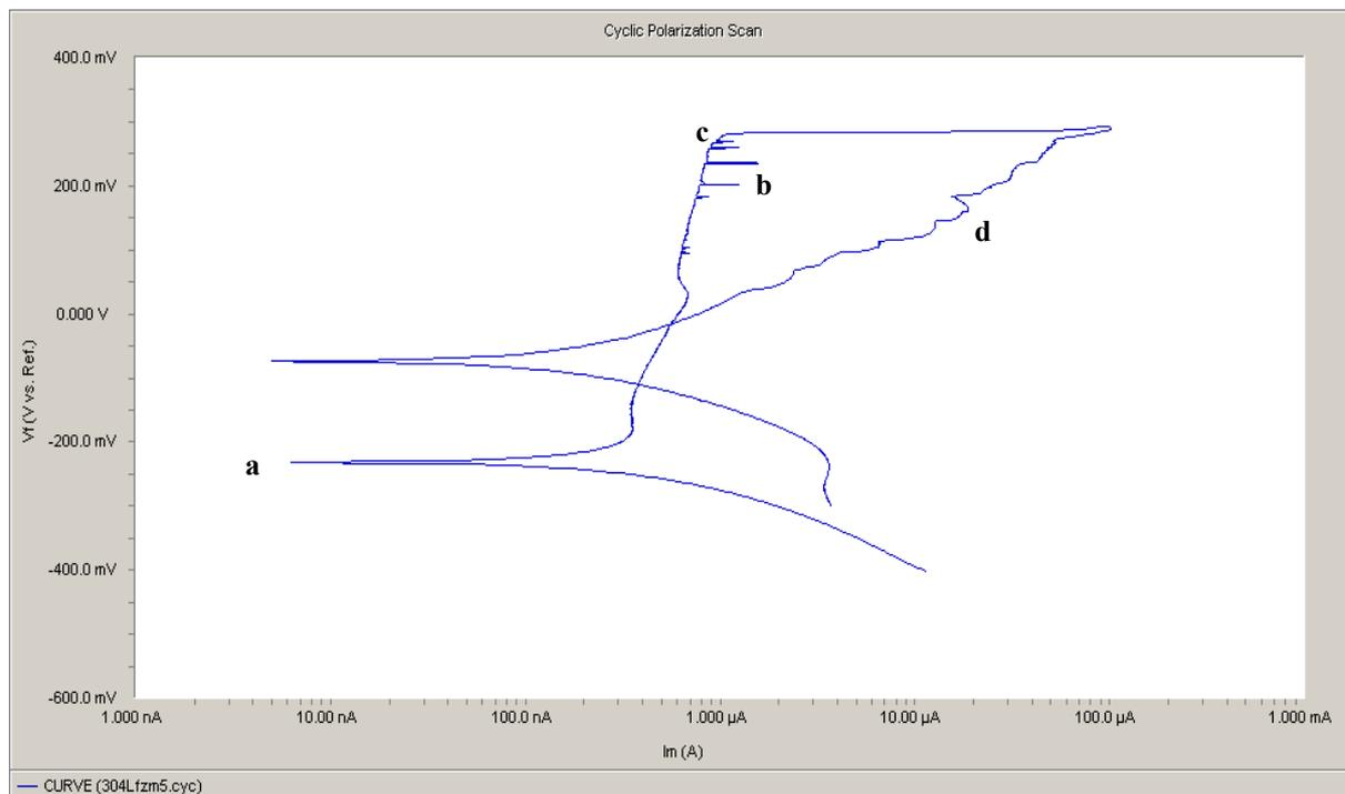
Fig. 6. Cyclic polarisation scan of the 304L polished sample in aqueous borate buffer solution containing 9g/L of NaCl, at room temperature. a) corrosion potential. b) electrochemical noise before pitting (depasivation / passivation cycles). c) pitting potential. d) return.
