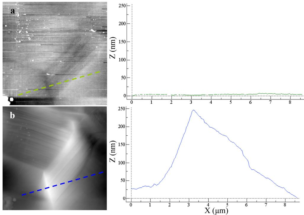
*Fig. 5. Topographic contact AFM images of the surface before (a) and after (b) high deformation rate (40% for b) and profiles drawn along the dashed lines. The blue profile shows different slopes from grain to grain after a high deformation: grain loosening has occurred.*
