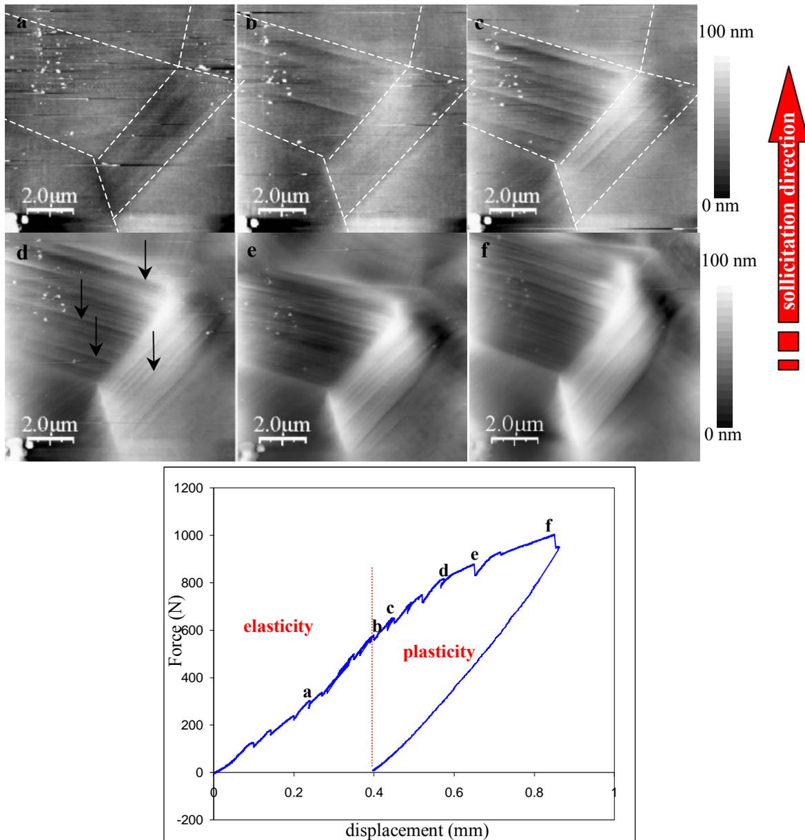
*Fig. 3. Topographic images of the same area during traction obtained in contact mode AFM and corresponding traction curve. The letters a,b,c,d,e,f correspond to different deformations in the traction curve. While a) is still in the elastic domain, b,c,d,e, and f belong to the plastic domain. At least 6 grains can be seen on the images, delimited here by dashed white lines. The arrows in d) point out the slip lines.*
