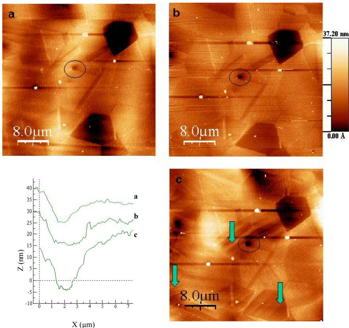
*Fig. 7. Evolution of the topography of the surface during traction (same traction curve than in air) at each step a, b and c. a) and b) are still in the elastic domain whereas c) is in the plastic one. The rings and the horizontal profiles corresponding show the pitting propagation of a pre-existent pit and the arrows show the slip lines in the grains. The z-scale is the same in all 3 images.*
