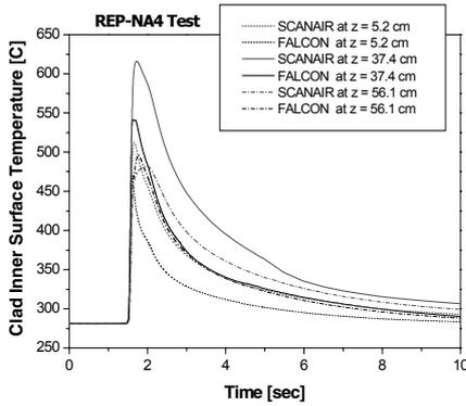
**Fig. 3:** Clad inner surface temperature predictions at three axial locations for REP Na-4.
