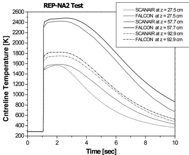
**Fig. 1:** Fuel centreline temperatures predicted by the codes at three axial locations for REP Na-2.
