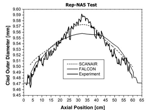
**Fig. 5:** Clad outer-diameter profile in REP Na-5 Test.
