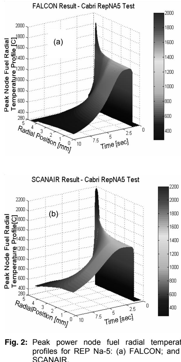
**Fig. 2:** Peak power node fuel radial temperature profiles for REP Na-5: (a) FALCON; and (b) SCANAIR.
