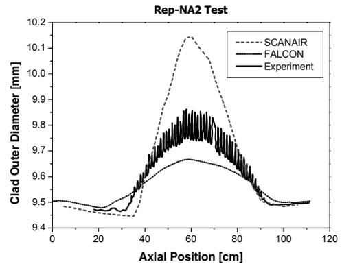
**Fig. 4:** Clad outer-diameter profile in REP Na-2 Test.
