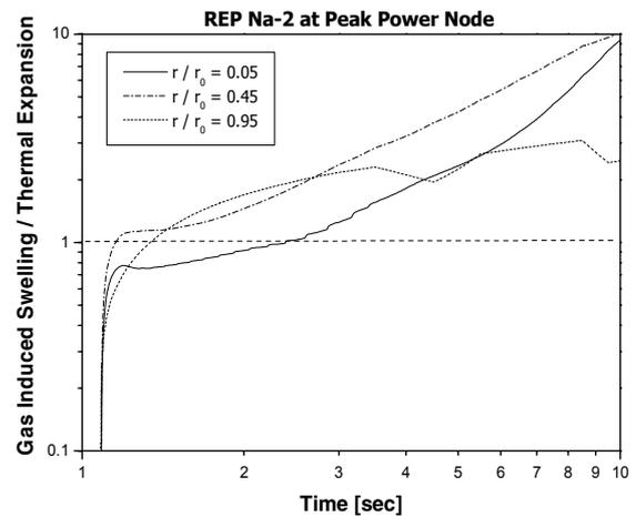
**Fig. 6:** Ratio of gas-induced to thermal fuel swelling at three different radial positions of the peak power node as calculated by SCANAIR for the REP Na-2 Test.
