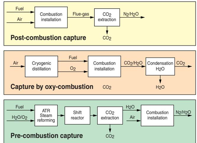
presence of water, or by partial oxidation in the presence of oxygen. The CO in the mix reacts with the water during the shift conversion stage to form CO<sub>2</sub> and hydrogen. Thus, the CO<sub>2</sub> is separated from the hydrogen under good conditions (precombustion capture) and the hydrogen can be used to produce energy (electricity or heat) without emitting CO<sub>2</sub>.
