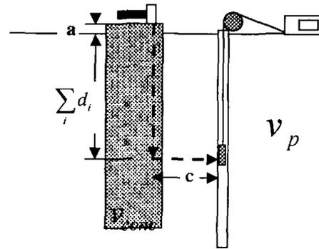
Figure 2: Travel path for the direct wave
