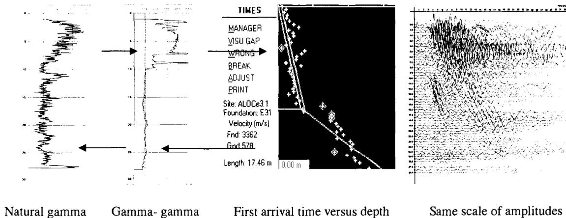
**Figure 6:** Combination of PSM and gamma logging for interpreting the evaluated depth
