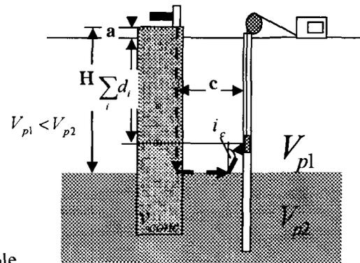
Figure 3: Travel path for refracted wave
