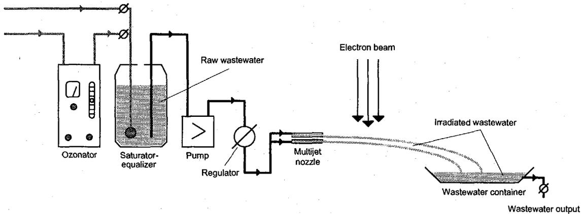
Fig. 1. Laboratory unit used in electron beam treatment experiments.
