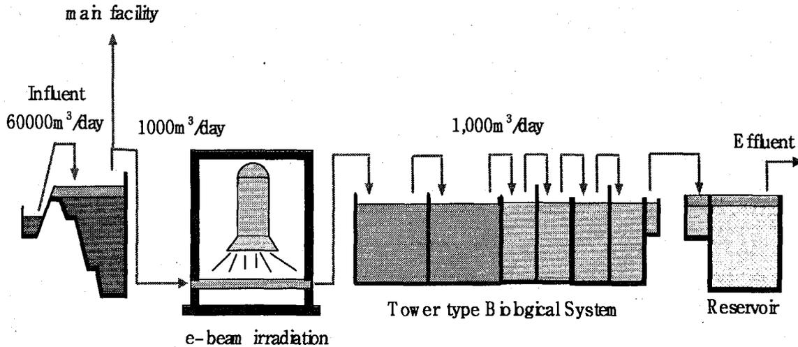
Fig. 6 Schematic Drawing of Pilot Plant
