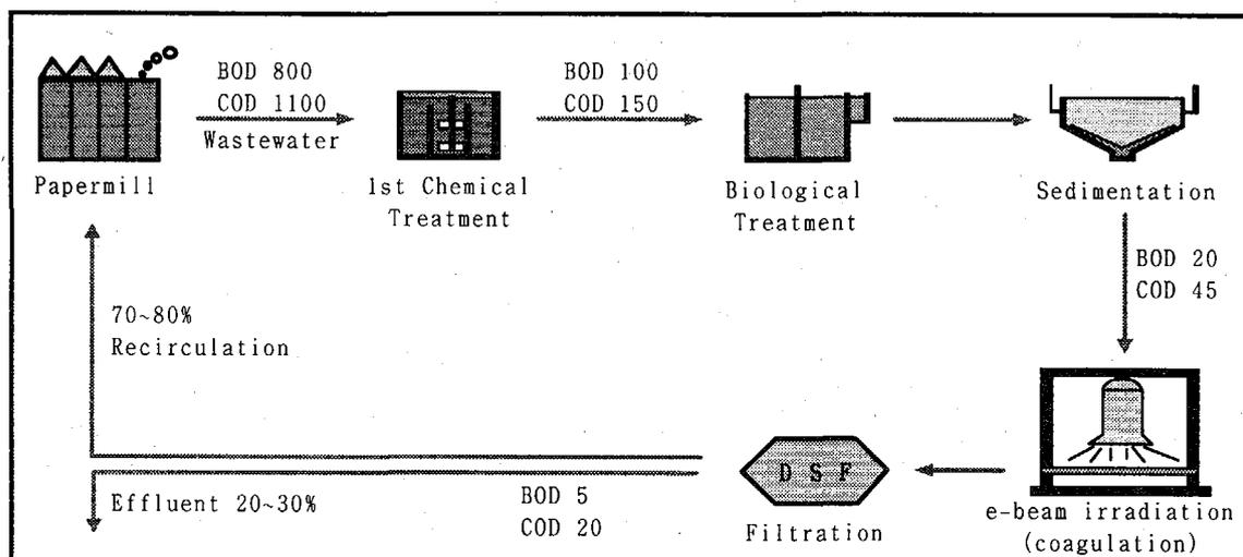
Fig. 3. Process flow of e-beam facility for wastewater from papermill.
