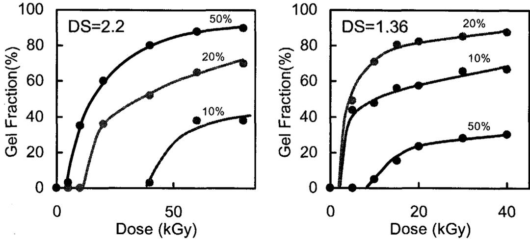
Fig. 1. Crosslinking of CMC by radiation
