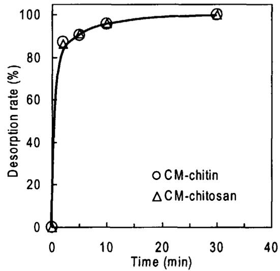
Fig. 5. Desorption kinetics of  $\text{Cu}^{2+}$  on crosslinked CM-chitin and CM-chitosan.
