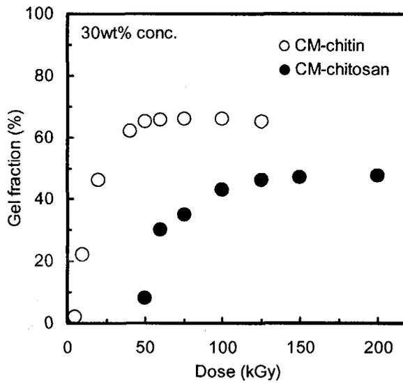
Fig. 3. Effect of irradiation dose on crosslinking of CM-chitin and CM-chitosan.
