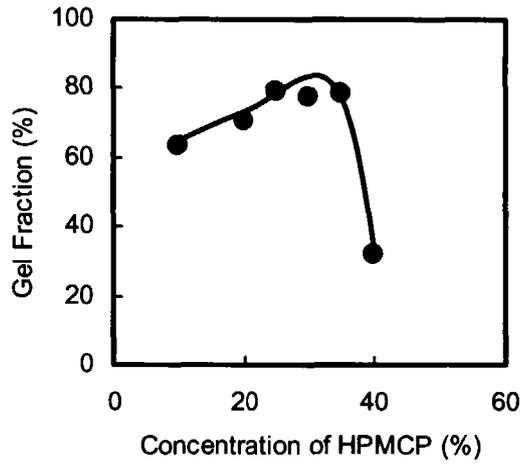
**Fig. 6. Radiation crosslinking of HPMCP in 5% Na<sub>2</sub>CO<sub>3</sub> solution.**
