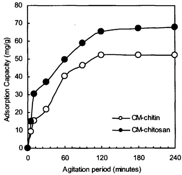
Fig. 4. Adsorption kinetics of  $\text{Cu}^{2+}$  on crosslinked CM-chitin and CM-chitosan.
